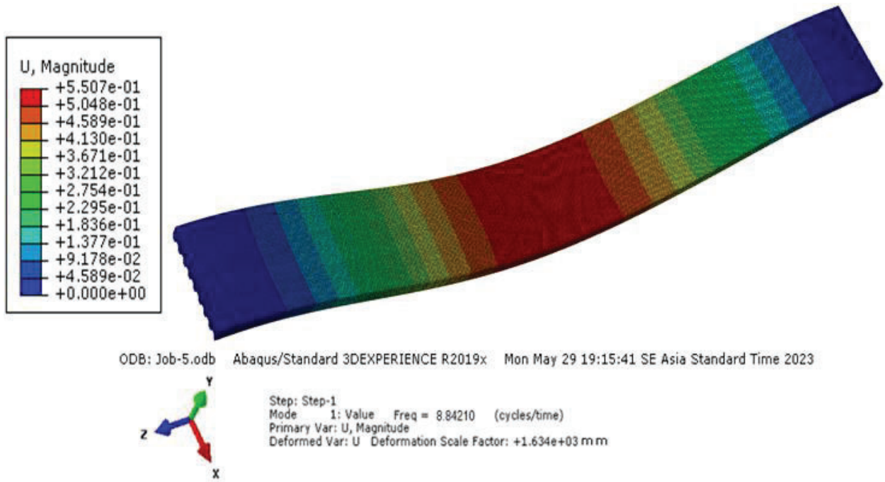
685 Fig. C3. Mode shape Frequency response of slab RCA100% slab for Model 3
