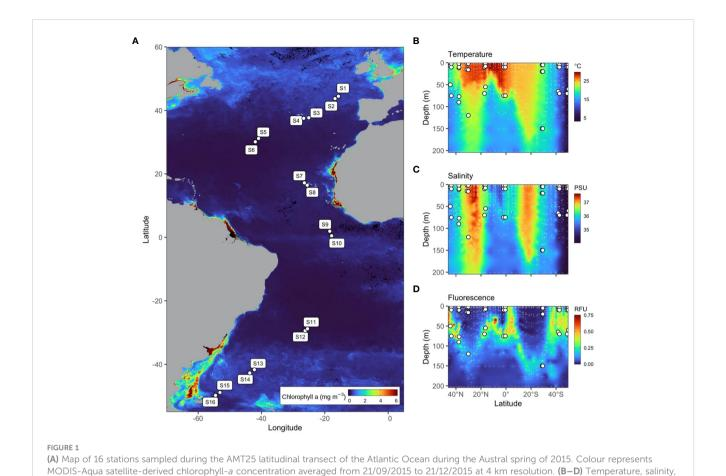
and fluorescence depth profiles throughout the Atlantic Ocean measured using the Sea-Bird SBE 911plus CTD and Aquatracka III Fluorometer,
