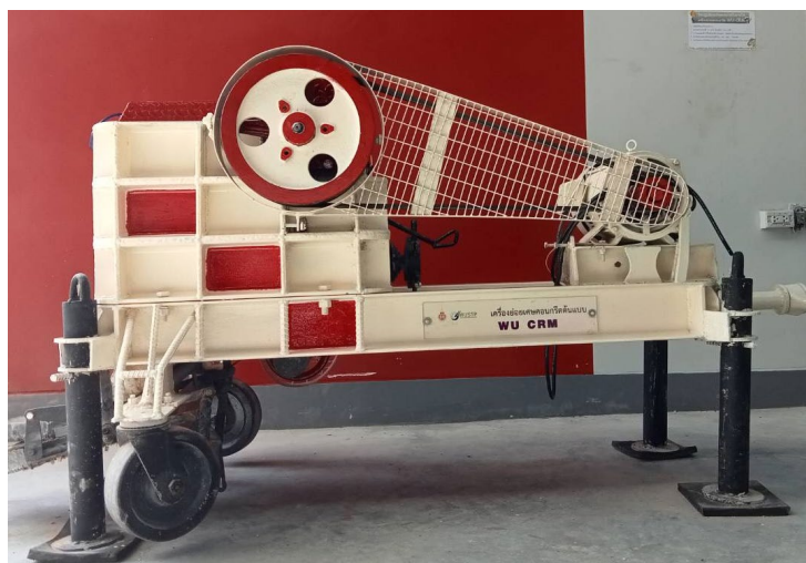
361 362 Fig. 5. Crusher machine used for concrete crushing
