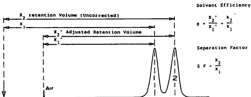
Figure 2 Calculation of solvent efficiency
