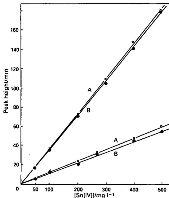
Fig. 2. Comparison of discrete volume nebulisation with direct uptake. A, Direct uptake to nebuliser; B, discrete volume nebulisation. Upper lines: acetylene at 2.2 l min<sup>-1</sup>, air at 5.0 l min<sup>-1</sup>; lower lines, acetylene 2.0 l min<sup>-1</sup>, air 5.0 l min<sup>-1</sup>
