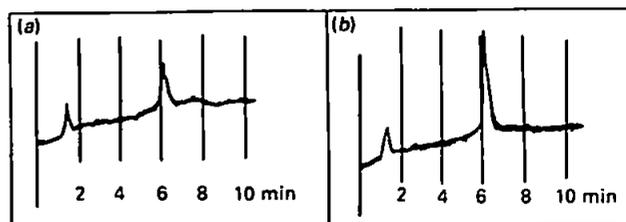
Fig. 6. Analysis of water samples collected at a harbour site in Plymouth, with and without co-injection of tributyltin chloride. (a) 1 ml of sample (800-fold pre-concentrated); (b) 1 ml of sample (800-fold pre-concentrated) + 500 ng of tributyltin chloride
