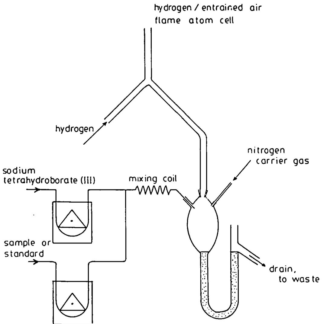
inlets, a fuel gas flow of  $180 \text{ ml min}^{-1}$  was used. The burner was then located vertically in the spectrometer, replacing the conventional burner/nebuliser assembly, and at the focal point of the entrance slit lens. The eluent from the high performance liquid chromatograph was introduced into the reaction manifold just prior to the introduction point of the tetrahydroborate (III) solution. The complete system is shown schematically in Fig. 31.
