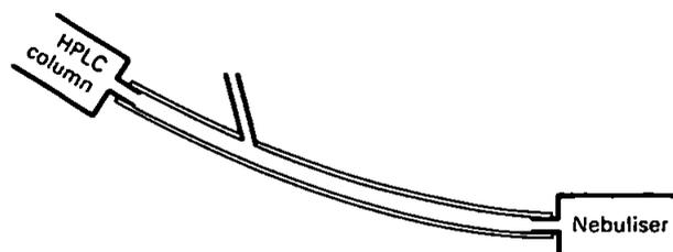
Fig. 1. Schematic diagram of HPLC - nebuliser interface
