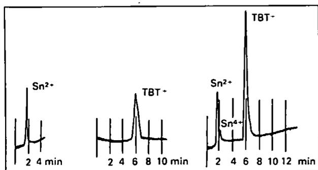
Fig. 5. Separation of tin species by coupled HPLC - FAAS
