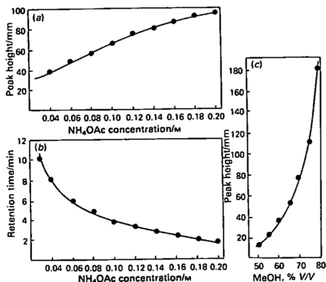
Fig. 4. Optimisation of chromatographic conditions. (a) Effect of ammonium acetate concentration on response for tributyltin ions; (b) effect of ammonium acetate concentration on retention time for tributyltin ions; and (c) effect of eluent composition on response for tributyltin ions
