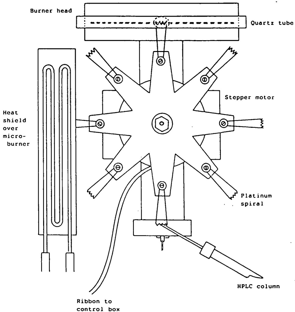
A plan view of the completed interface is shown in Figure 55.
