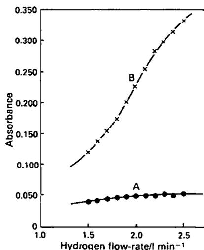
Fig. 3. Effect of changing the hydrogen flow-rate when using the slotted-tube atom trap and an air-hydrogen flame for (A) tin(IV) solutions and (B) tributyltin chloride in 20% methanol
