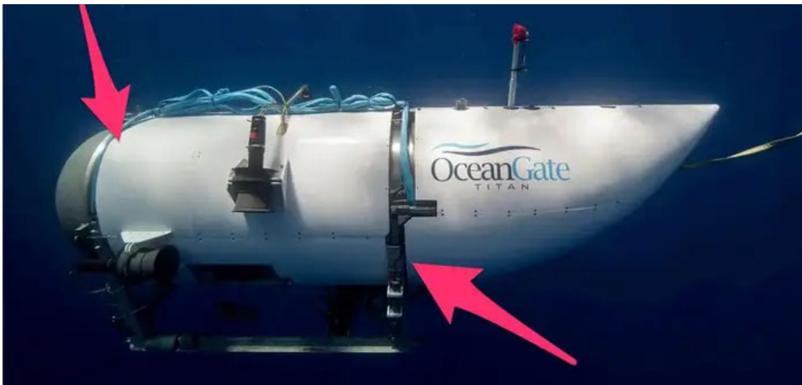
An annotated picture points to the approximate location of the structural titanium rings. OceanGate Expeditions/Reuters/Insider
