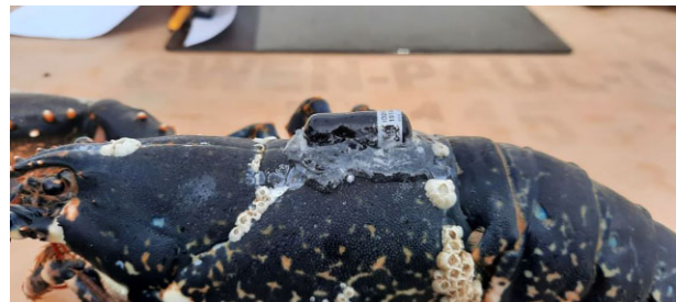
Figure 2. Innovasea V9 acoustic transmitter attached to carapace of European lobster ( H. gammarus ) using cyanoacrylate glue and epoxy resin.
