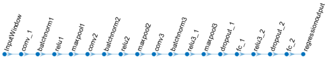
Figure 3. Deep neural network structure implemented using MATLAB deep learning toolbox.
