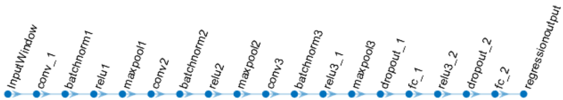
Figure 3. Deep neural network structure implemented using MATLAB deep learning toolbox.
