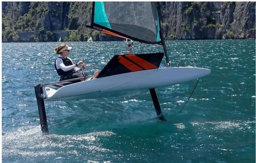
Skeeta using fully articulated balanced foils
