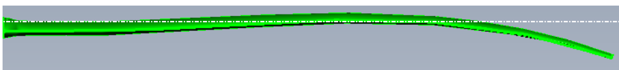
Balanced ‘Gull Wing’ foil with foil drag balanced above and below the pivot axis
