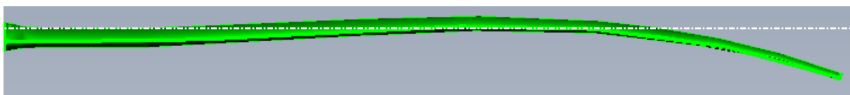
Balanced ‘Gull Wing’ foil with foil drag balanced above and below the pivot axis
