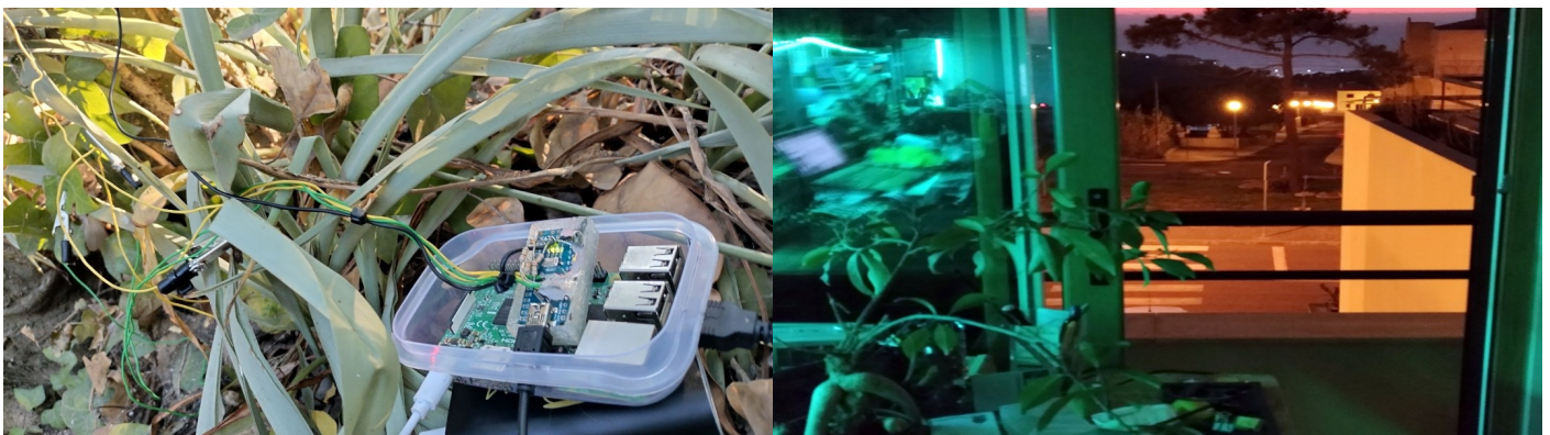
Figures 126, 127: Portable bio-electric voltages sampling device made with C++ code, Arduino pro with electronics for 6 analog sampling channels being logged on a rPI 3B+ used to field capture bio data; Precursor bio-data acquisition from my currently 16 years old bonsai tree during 2018.
