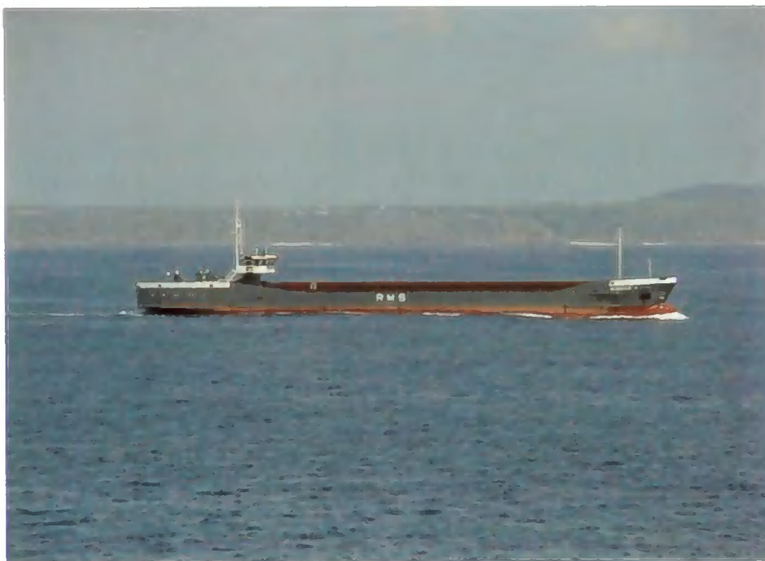
Figure 6-13 River-sea ship with hydraulic wheelhouse
