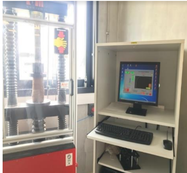
Figure 4. Compressive strength test on cob samples at different water content under an IGM press.
