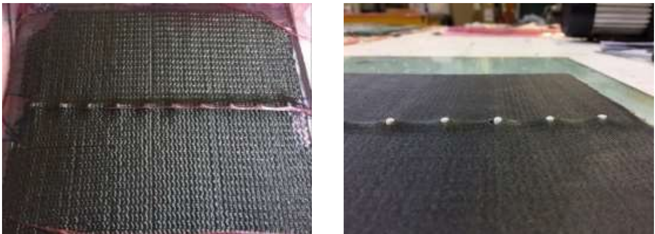
Figure 15: Left: bridging of vacuum bag, right: resulting raised sections around holes.
