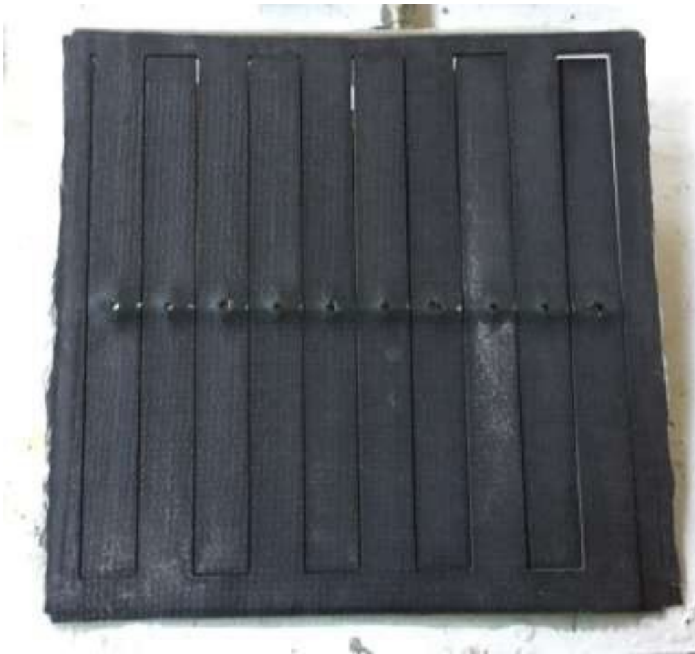
Figure 8: Moulded plate once waterjet cut, note continuous profile leaving one uncut edge.
