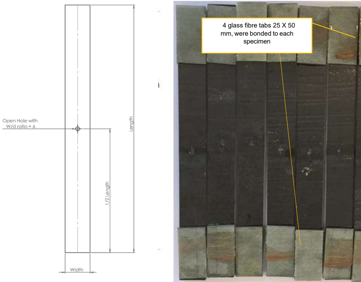
Figure 12: Left: schematic of open-hole tensile test specimen, right: annotated actual samples.
