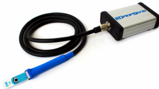
Figure 2.6: A \mu Stat BiPotentiostat/Galvanostat and a screen printed disposable electrode, both from Dropsens (Spain). The potentiostat is used to maintain the working electrode's potential at a constant level and adjusting the current. The electrode is a three electrode system printed on a substrate and can be connected to the potentiostat. The principles are explained in section 1.4.1.
