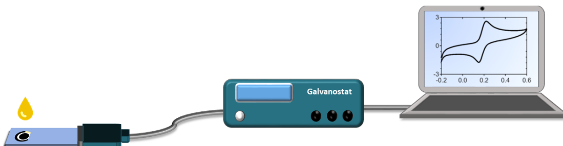
Figure 2.7: A schematic of a measurement setup, using a galvanostat and a software interface.
