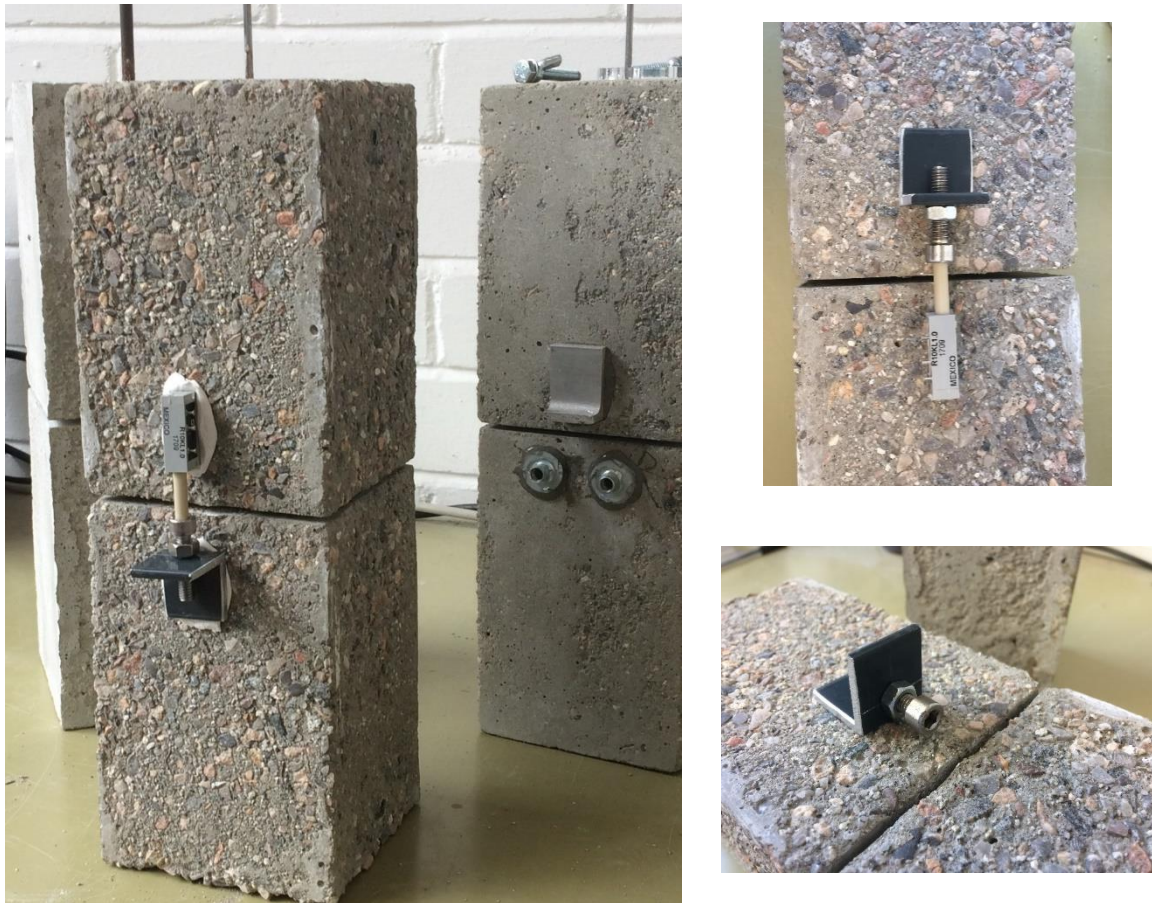
Figure 5.5 Displacement sensor arrangement (Source: Nirvan Razaghi-Kashani).
