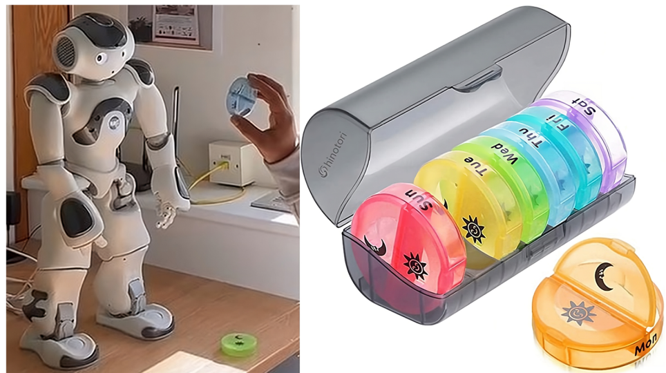
Fig. 2 Demonstration of the real experimental setup of the humanoid robot NAO (left) recognising the coloured fictional supplement boxes (right), by means of the interfaced YOLOv5 object recognition module
