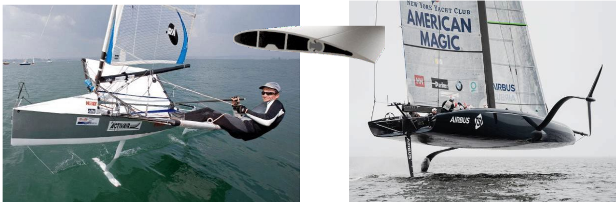
Moth and AC75 are particularly efficient, using flapped foils
