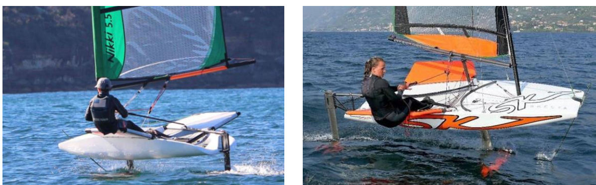
Nikki and Skeeta foiling dinghies use an active balanced foil system
