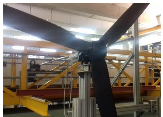
Figure 3: CFRP FLOW turbine blades installed in the University of Plymouth COAST Laboratory
