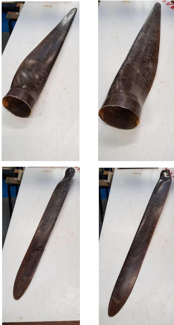
Figure 8: Four views of the completed FLOW turbine blade
