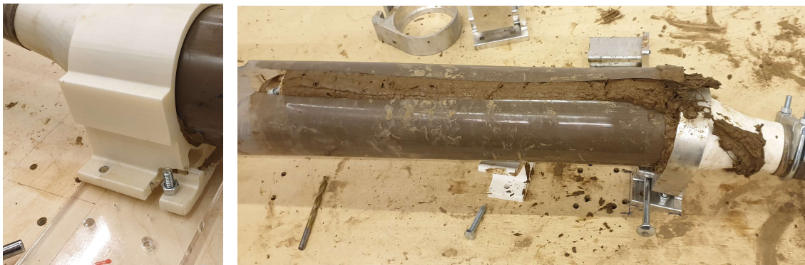
Figure 11. Destruction of the 3DP PLA joints due to pressures caused by the cob mix (left) and the destruction of the cartridge due to pressures caused by the bending plywood platform (right).
