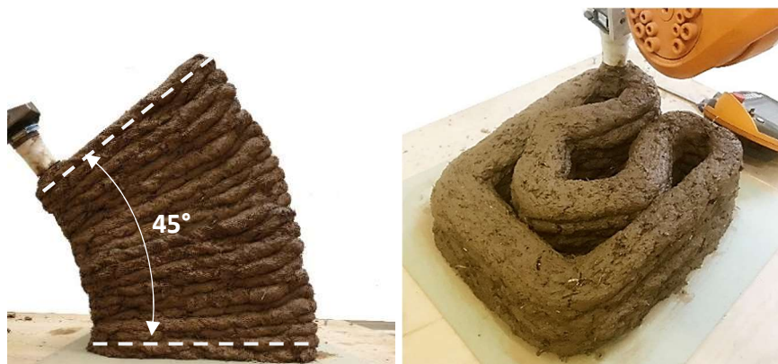
Figure 25. Testing complex movement through 3D printing arch-based geometry.
