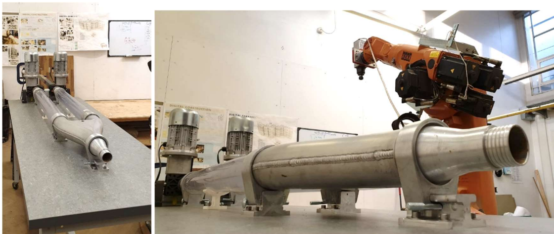
Figure 13. Scheme of the new bespoke dual extruder components: 1) Screw jack, 2) Cob Cartridge, 3) Steel-wired PVC hose, 4) Nozzle, 5) Aluminum parts, 6) Mobile platform, 7) Cartridges Rack.
