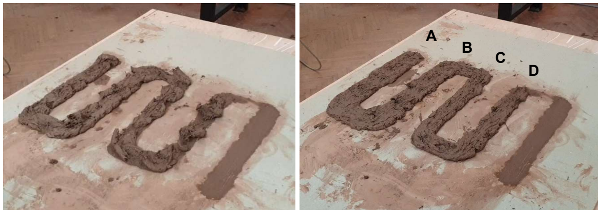
Figure 18. Explorations of the synchronization process between extrusion rate and robot motion speed (left & right)
