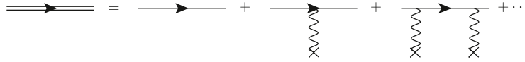
Fig. 4. The diagrammatic expansion of the Furry picture propagator in terms of ordinary (position space) Feynman diagrams in vacuum; each external photon line represents an interaction with the external field via the usual vertex -ieA_\mu\gamma^\mu .
