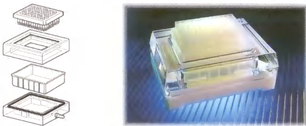
Figure 1.31: Diagram (3M, 1998) and photograph (Varian, 2000) of a 96 well plate.
