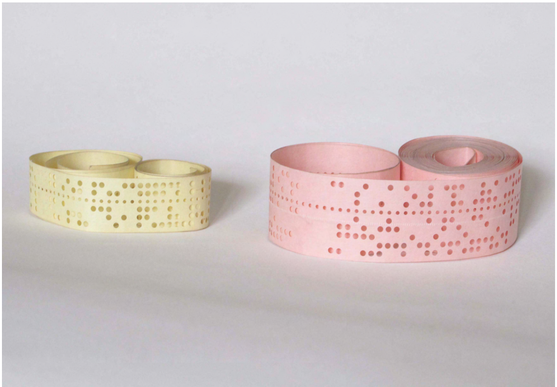
Figure 64: Early five- and eight-hole punched computer tape (Coles, 2010).
