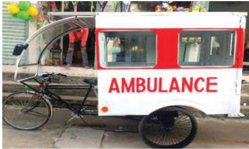
Figure 2.4 Solar Electric Ambulance Van (Tarek et al. , 2016) Permission to reproduce this extract has been granted by © 2016, IEEE
