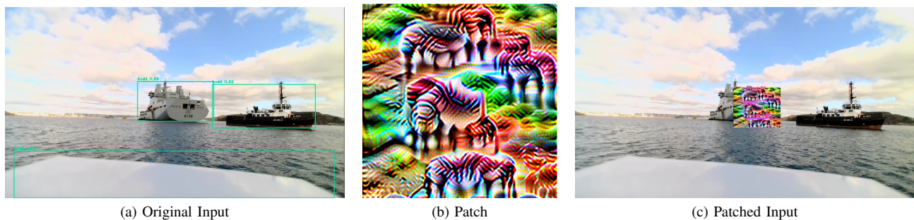
Fig. 4: A real-world adversarial patch attack sample [43] generated to attack the common pre-trained YOLOv3 object detection model. The input sample, an image of two vessels, is predicted as a vessel by the model, providing a confidence value of 99% and 92%. An adversarial patch (b) is provided digitally or physically (e.g., as a sticker) to change the detection prediction to a zebra by the model. Notice the patch can interfere with the prediction and hide nearby objects, such as the second ‘boat’, i.e. vessel, on its right in the photo. The patch does not need to be significantly large but can be closer to the camera than the evading objects to produce the desired effect.
