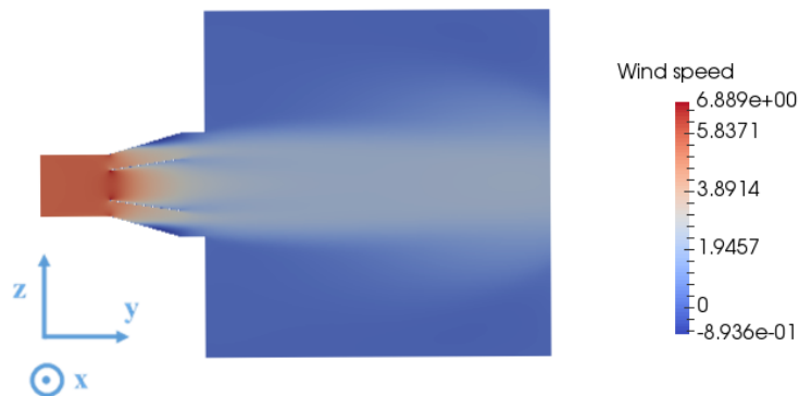
Figure 4.43: Cross section parallel to the main direction of the flow for a 1.8 m diameter inlet using 6 subdivisions and an inner cones measuring 1/2 of the outer diameter
