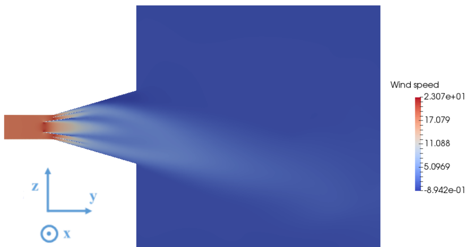
Figure C.5: Wind speed in slice parallel to the main direction of the flow
