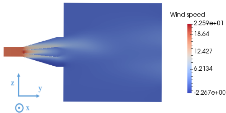
Figure 4.37: Cross section parallel to the main direction of the flow for the diffuser with a 1 m inlet diameter and a long inner cone with a diameter measuring a 1/3 of the outer diffuser. No subdivisions were used
