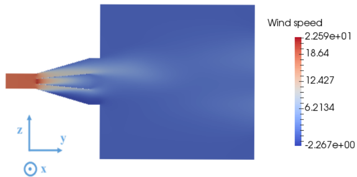
Figure C.17: Slice parallel to main direction of flow
