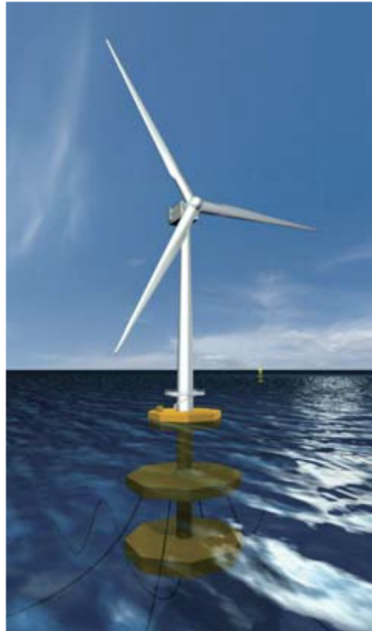
Figure 2.4: Advanced SPAR concept used for Fukushima Hamakaze (5 MW), taken from Ishihara et al. (2014) with the permission of T. Ishihara
