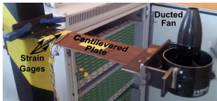
Figure 2.26: Measurement of thrust produced through ducted fan by means of a sheet metal and strain gauges, reproduced from Wright et al. (2015a) with the permission of MARINET
