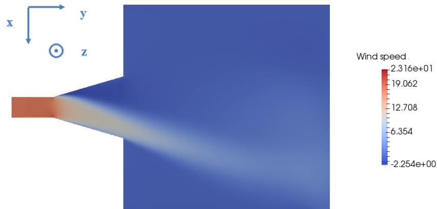
Figure C.1: Wind speed in slice parallel to the main direction of the airflow
