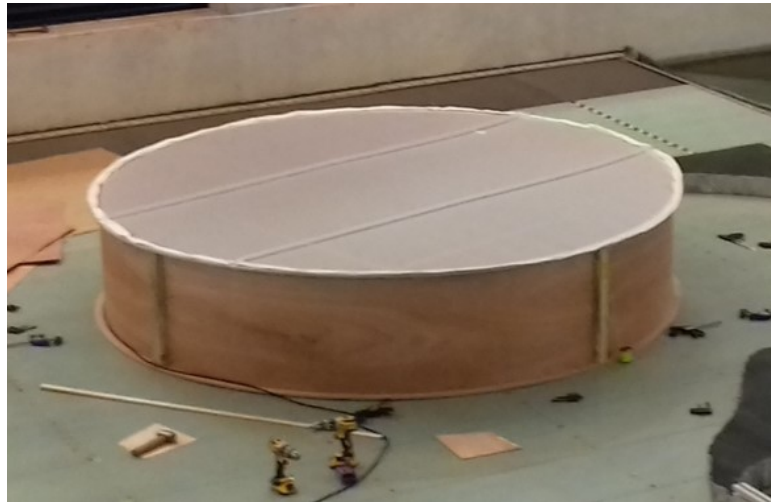
Figure 5.37: Short straight cylindrical section holding the meshed screen (visible) and the honeycomb in place (hidden)
