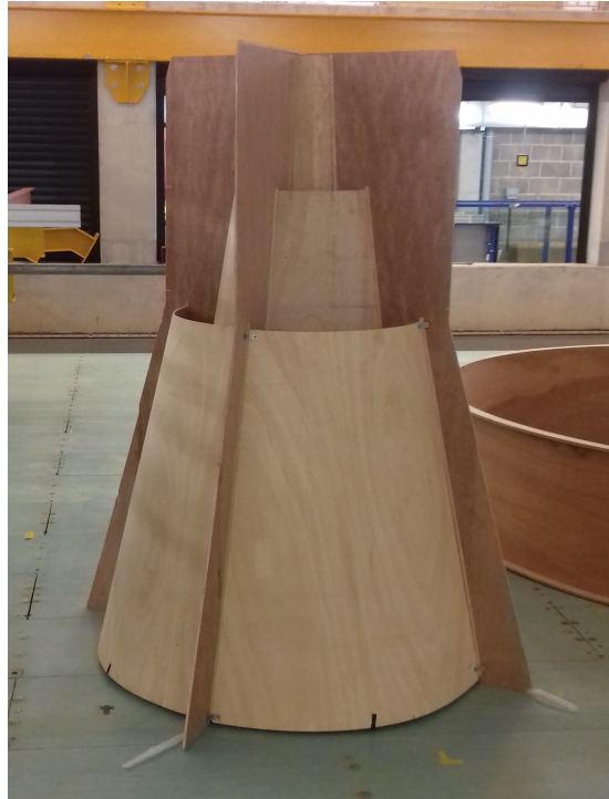
Figure 5.22: Set of nested concentric cones situated inside the diffuser cone
