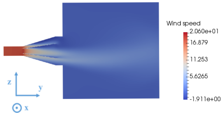
Figure 4.41: Cross section parallel to the main direction of air flow for a diffuser with a 1 m inlet diameter and a long inner cone with a diameter measuring a 1/2 of the outer diffuser. No subdivisions were used
