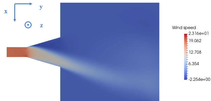
Figure 4.32: Wind speed in slice parallel to the main direction of the airflow
