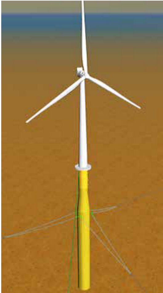
Figure 2.3: Hywind SPAR buoy platform (taken from EWEA-WindEurope (2013) with the permission of WindEurope (formerly EWEA))
