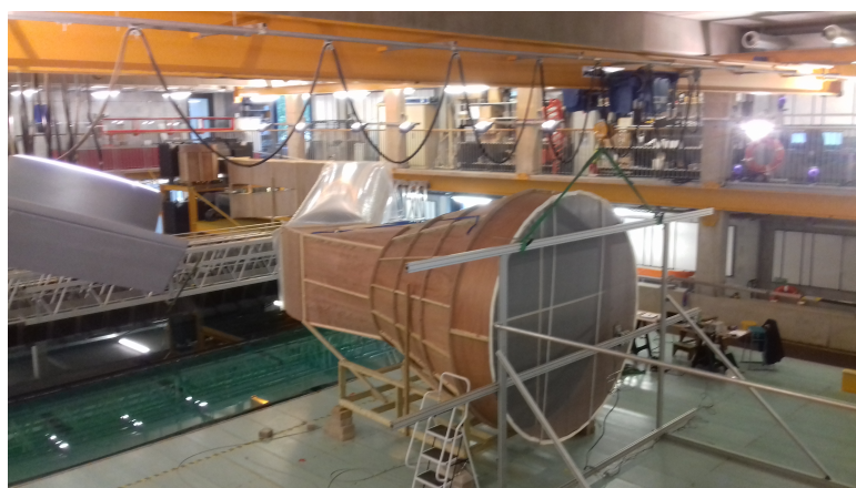
Figure 5.51: Ducting system from fans to outlet
