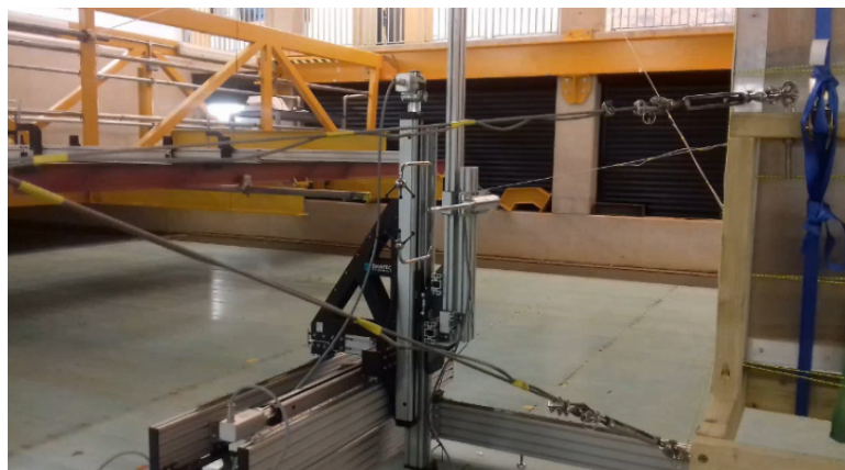
Figure 5.11: Traverse and anemometer used to measure the wind at various positions near the outlet
