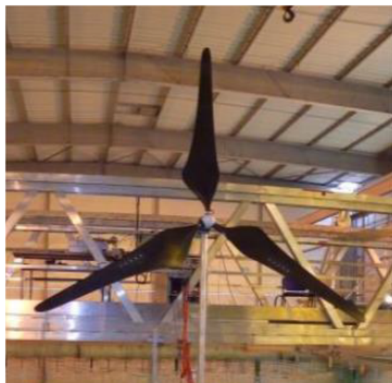
Figure 2.46: Low Reynolds rotor used by Sandner et al. (2014), with the permission of F. (Sandner) Lemmer
