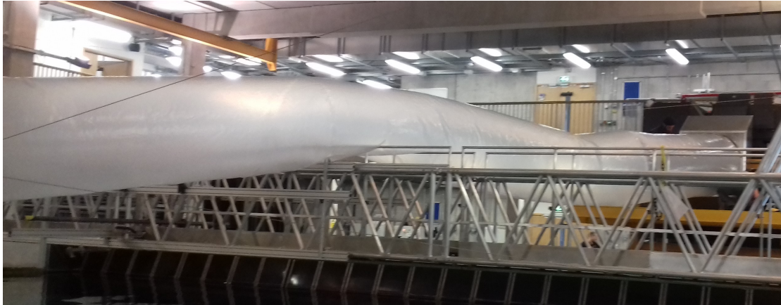
Figure 5.10: Polythene duct that guides air from fans to outlet situated at the centre of the basin
