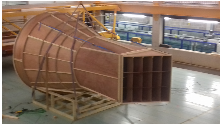
Figure 5.49: Diffuser cone in centre of basin with second set of guide vanes
