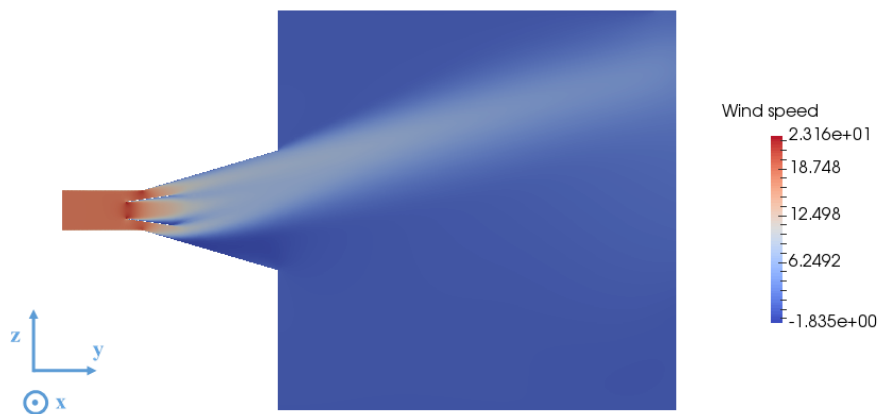
Figure C.15: Wind speed in slice parallel to the main direction of the air flow
