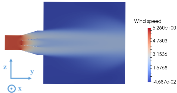
Figure 4.39: Cross section parallel to the main direction of the flow for the diffuser with a 1.8 m inlet diameter and a long inner cone with a diameter measuring a 1/3 of the outer diffuser. No subdivisions were used
