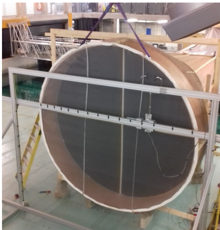
Figure 5.38: Diffuser cone with flow straighteners installed and structure to hold anemometer for measurements
