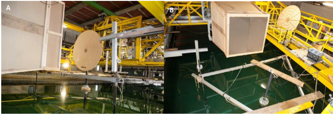
Figure 2.30: Drag disc experiments at CNR-INSEAN, Rome, Italy. Found in Wright et al. (2015a), originally from (Wan et al., 2014b). Permission obtained by MARINET
