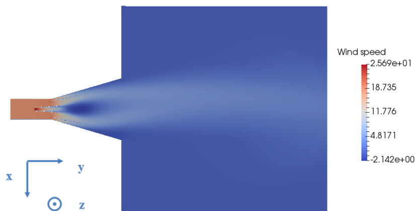
Figure C.13: Wind speed in slice parallel to the main direction of air flow
