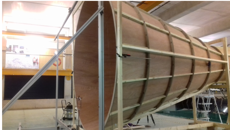
Figure 5.21: Truncated cone diffuser
