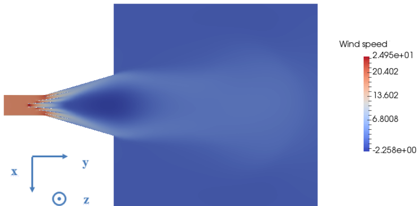
Figure C.3: Wind speed in slice parallel to the main direction of the airflow
