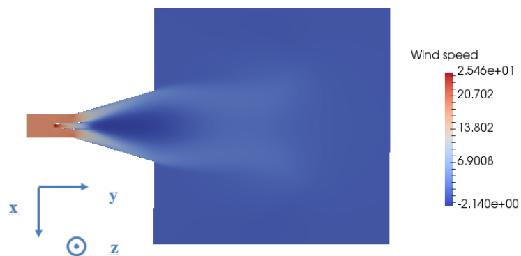
Figure C.11: Wind speed in slice parallel to the main direction of air flow
