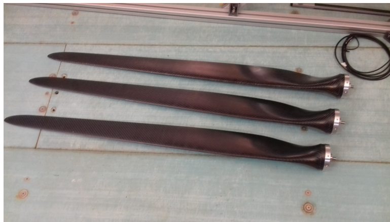
Figure 6.8: Wind turbine blades
