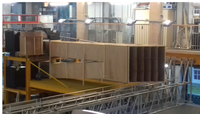
Figure 5.48: Structure near fans including wooden structure to combine air flow of the two fans and first set of guide vanes
