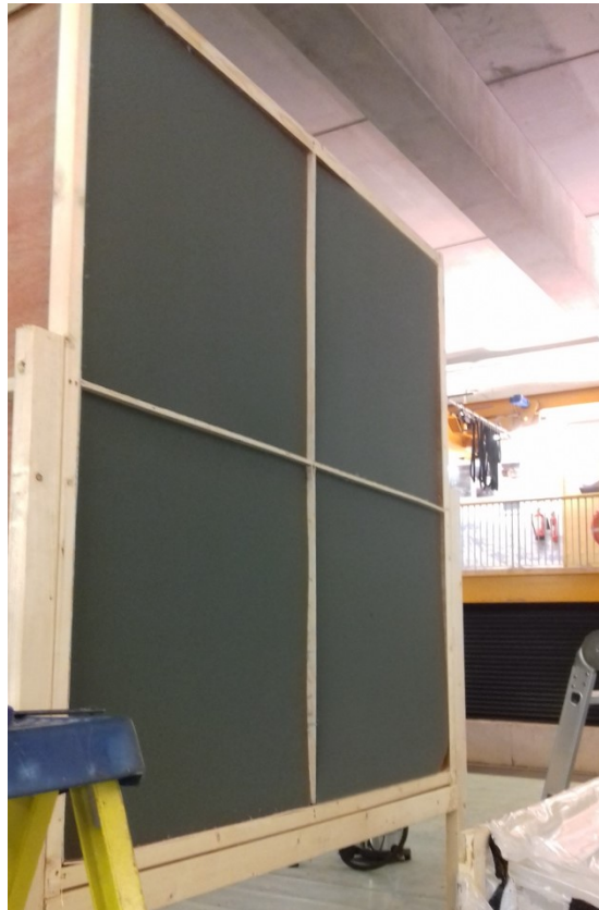
Figure 5.36: Honeycomb upstream of diffuser cone
