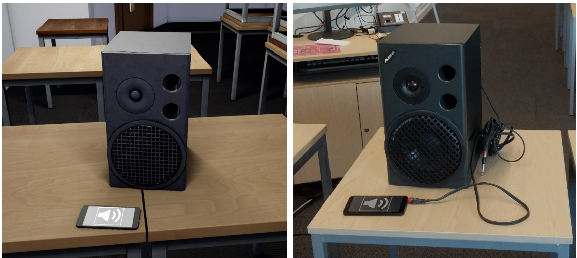
Figure 4.2: Above images show the speakers that deliver the word lists (left – Virtual World, right – Real World). Participants would tap the mobile phone screen in front of the speaker to activate the word lists.
