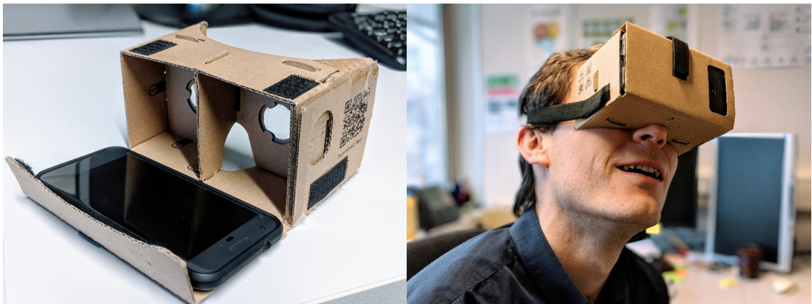
Figure 2.3: (Left) Shows how a mobile phone is placed as the display for Google Cardboard head-mounted display. (Right) Shows the placement of the Google Cardboard display in use.
