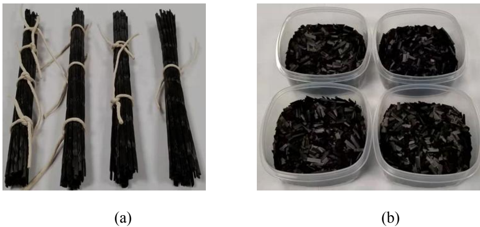
Fig.4-16 A set of four groups of CFS samples used for the water uptake test: (a) 240 mm long strands; (b) 6 mm short strand.
