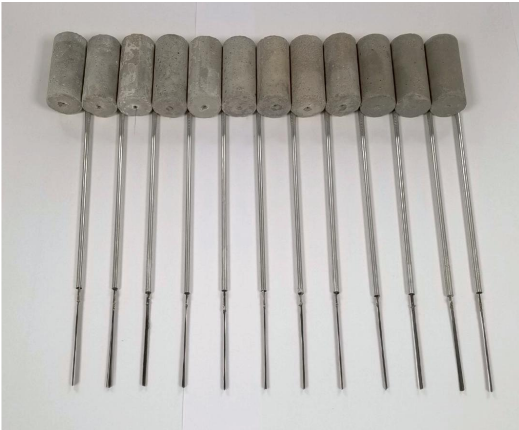
Fig.6-3 Tested CFSRM specimens exposed to elevated-temperature accelerated ageing of seawater immersion at 60 °C.
