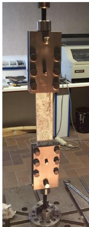
Fig.2-14 Tensile test of a plate sample after ageing treatment (Munck et al., 2018).
