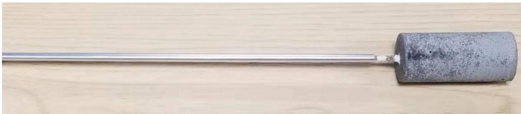
Fig.4-22 The completed CFSRM specimen for the pull-out test.
