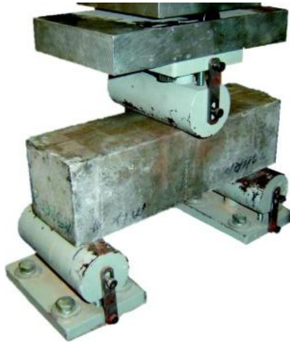
Fig.2-17 Bending test of FRP reinforced beam after ageing treatment (Tatar and Hamilton, 2016).
