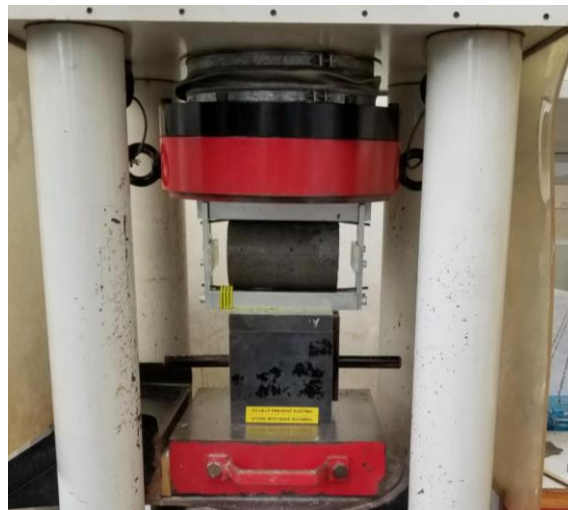
Fig.4-5 The splitting tensile test of mortar cylindrical specimen.
