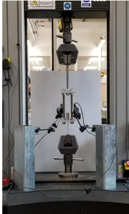
Fig.4-24 Pull-out test setup.
