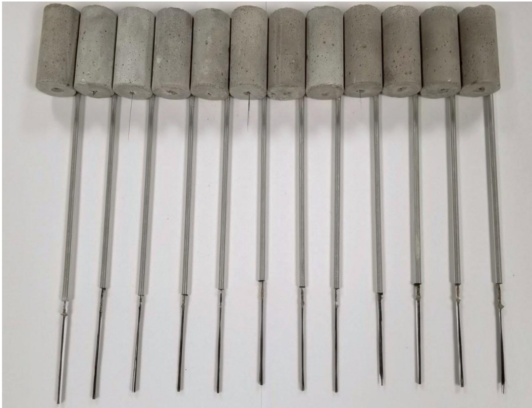
Fig.6-8 Tested CFSRM specimens exposed to the normal service condition of seawater immersion at 20 °C.
