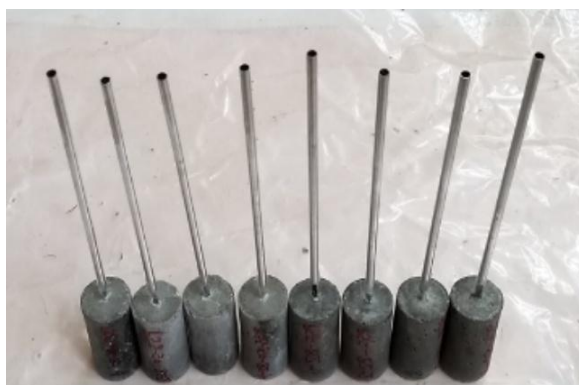
Fig.4-25 Samples used for static pull-out test: seawater batch (PI-1, 2, 3, 4) and freshwater batch (PI-1F, 2F, 3F, 4F).
