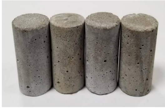
Fig.4-10 A set of four SM specimens used for the water uptake test.
