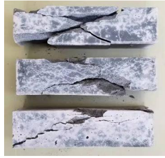
Fig.4-27 Tested specimens of mortar uniaxial compressive elastic modulus test.
