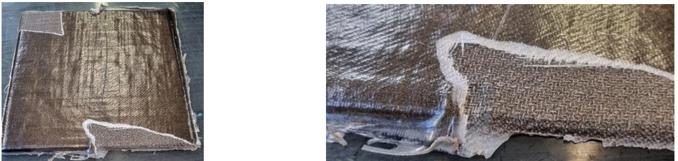
Figure F4: The cured laminate after attempting to remove the peel ply at panel scale (left), and detail of a corner (right).
