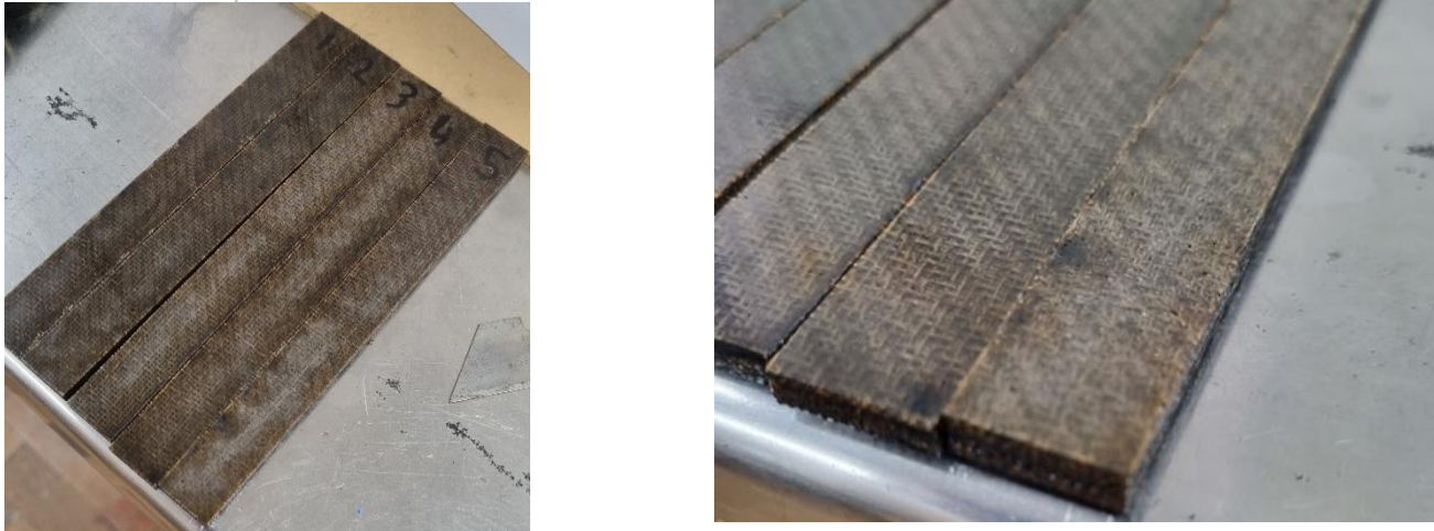
Figure F5: Test samples extracted from the NFM/PP laminate by laser cutting (left) and close-up (right) indicating an extremely low surface breaking void volume.
