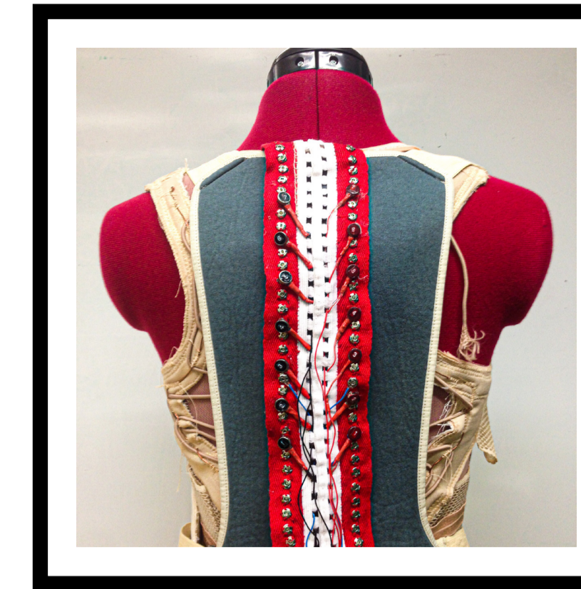
Figure 1. Haplós attached to a modified, commercially-available back support garment.
