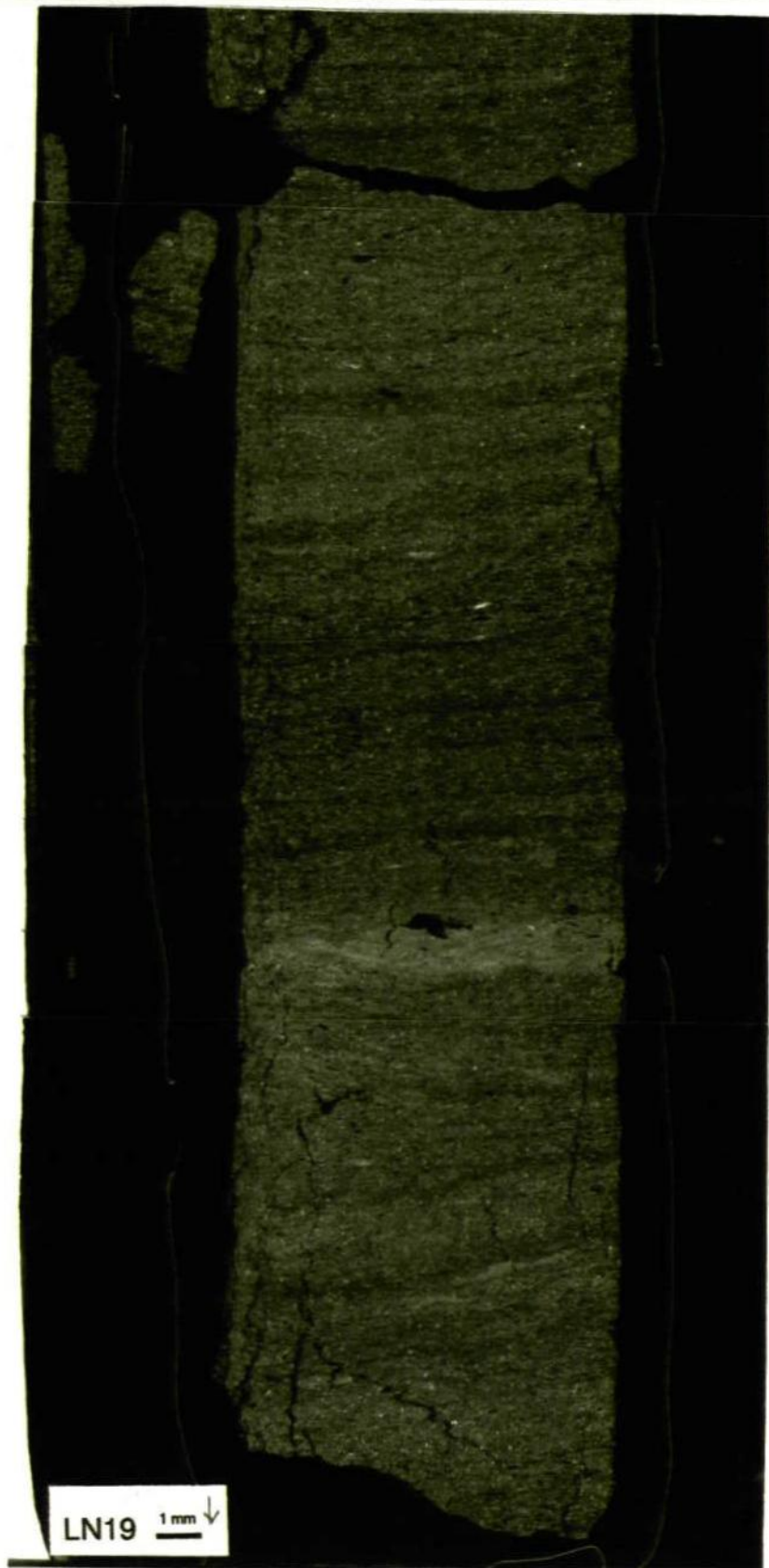
Plate 6.1 A photomosaic BSEI image of a section from core Ness 4 . The sediment is of Mid-Holocene age ( J.M. Dean, pers. comm. ).
