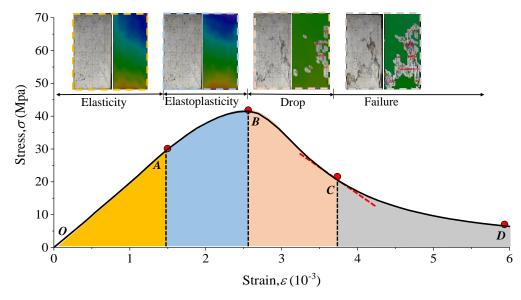
Fig. 6 The typical axial compression stress-strain curve
