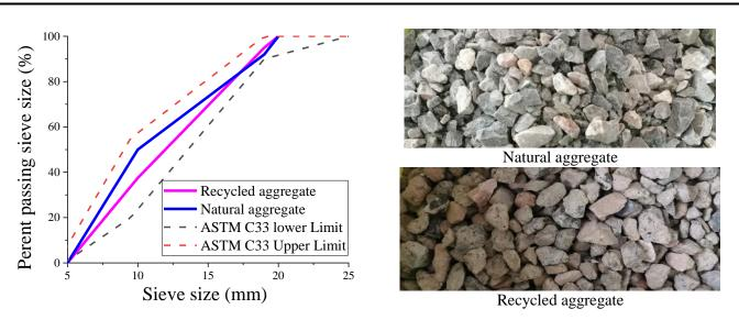
Fig. 1 Particle size distribution curve of aggregates and their appearance
