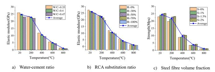
Fig. 10 Elastic modulus of concrete samples versus temperature
