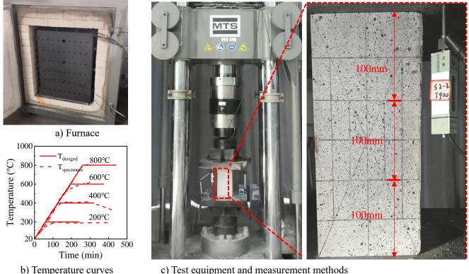
c) Test equipment and measurement methodsFig. 3 Heating and loading processes
