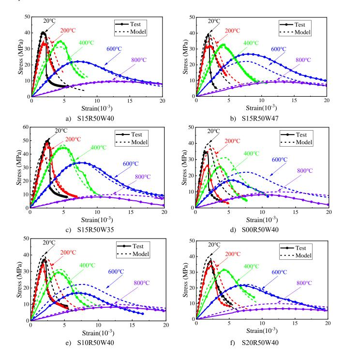
less brittle when the exposed temperature increases because of the formation of thermal cracks at high temperature environment.
