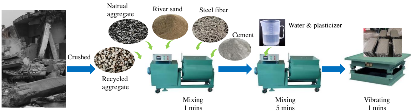
Fig. 2 The process of fabrication of tested specimens
