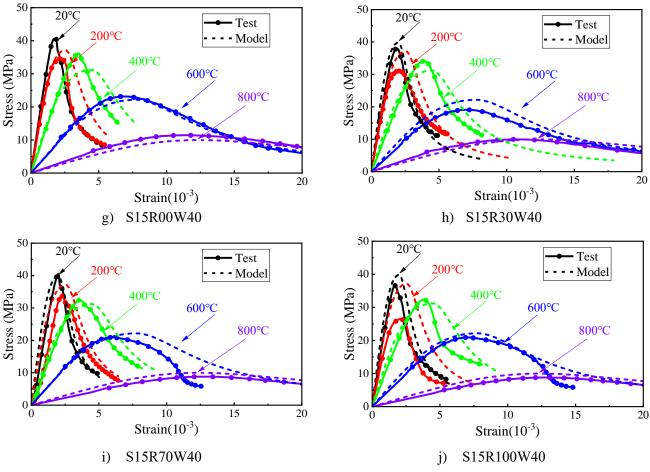
Fig. 5 Comparison between the stress-strain curves from experiments and the proposed model
