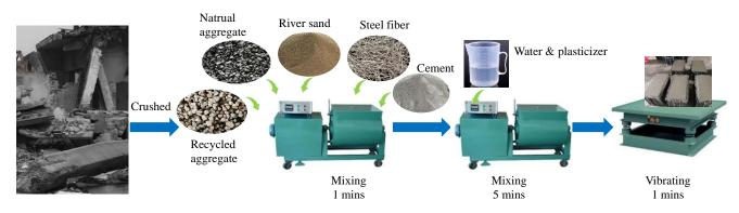
Fig. 2 The process of fabrication of tested specimens
