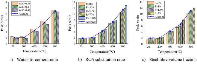
Fig. 12 Peak strain of concrete samples versus temperature
