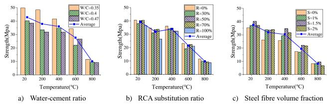
Fig. 8 Compressive strength of concrete samples versus temperature
