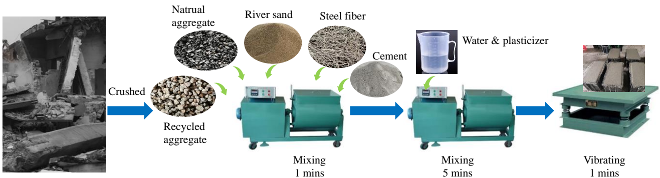
Fig. 2 The process of fabrication of tested specimens
