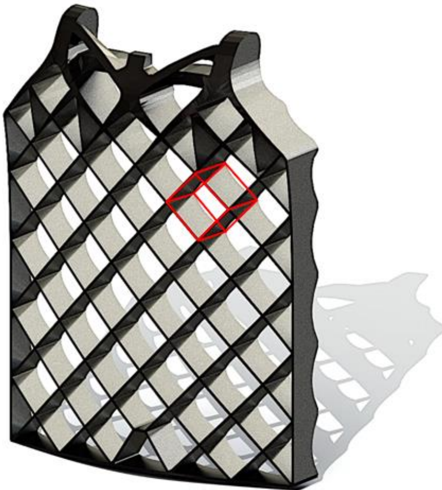
Figure 25: Cell study geometry in the context of grid fin
