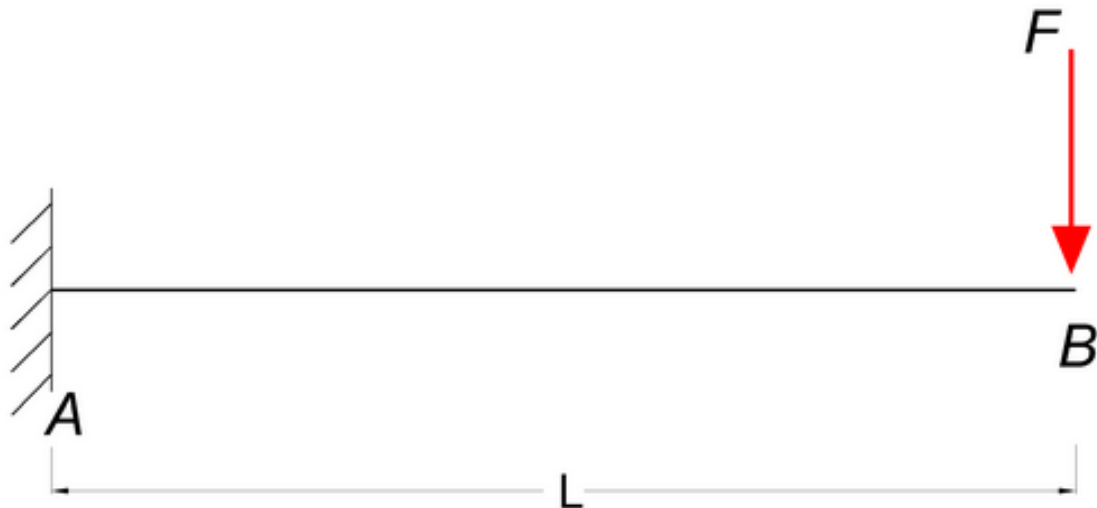
Figure 36: Cantilever beam schematic, point load
