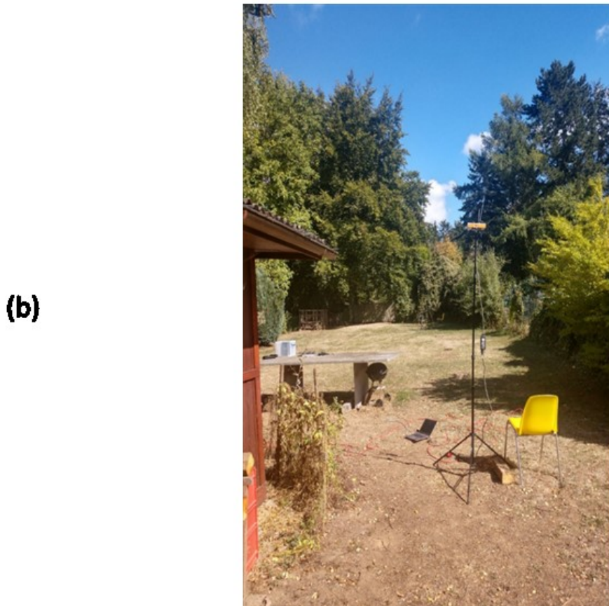
Figure 5.1: (a) Sensibility of the WLE600VX WLAN module, IEEE802.11n, 20MHz (Compex Systems, 2021), (b) Mini-PC on tripod during measurements of WLAN transmission and interference range
