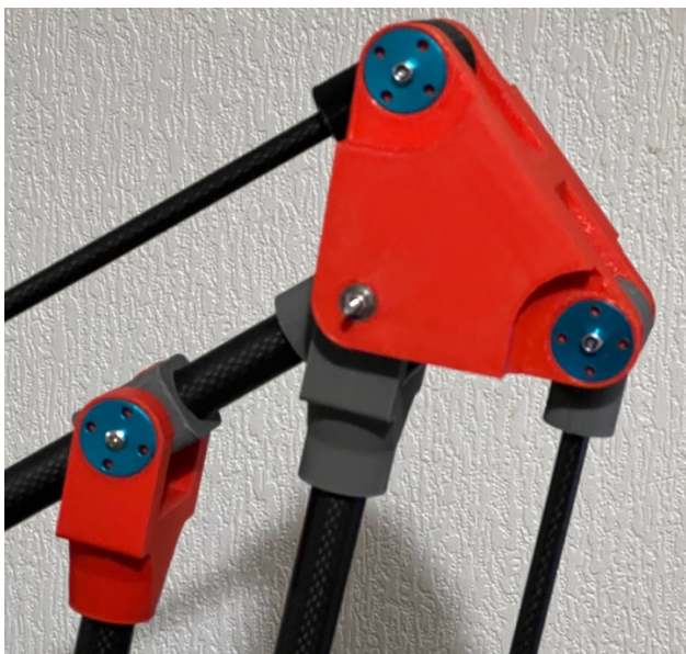
Figure 3. 2D arm. Endpoint alignment joint mechanism. A triangular mechanism is used to transfer motion of the passive arm to ensure the end effector always remains at a constant angular orientation.
