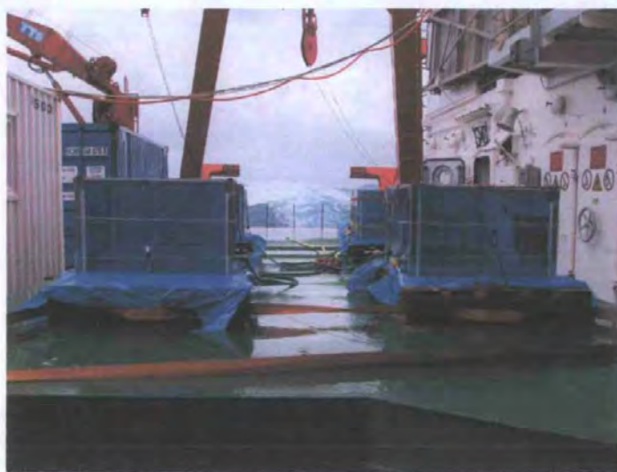
Figure 3.3 On deck incubator tanks used during dissolution studies. Light was attenuated to 20% of incident surface values using blue filters.
