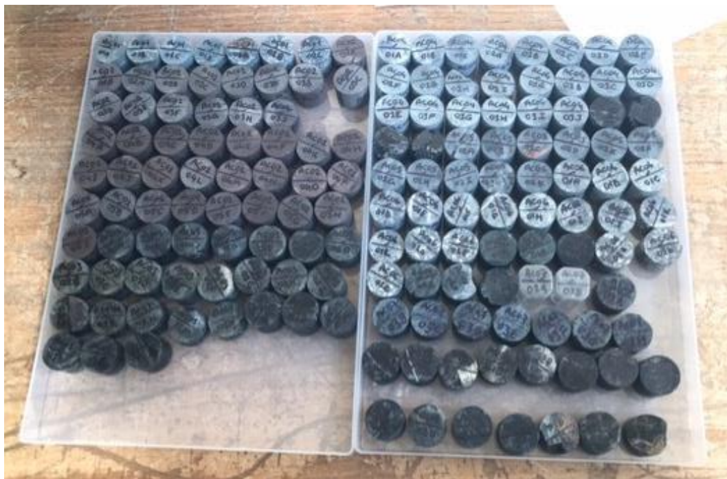
Figure 3.18. An image of the specimens were used for this study. They are basalt, dolerite, gabbro, lavas, serpentinite, and siltstones. They are numbered.
