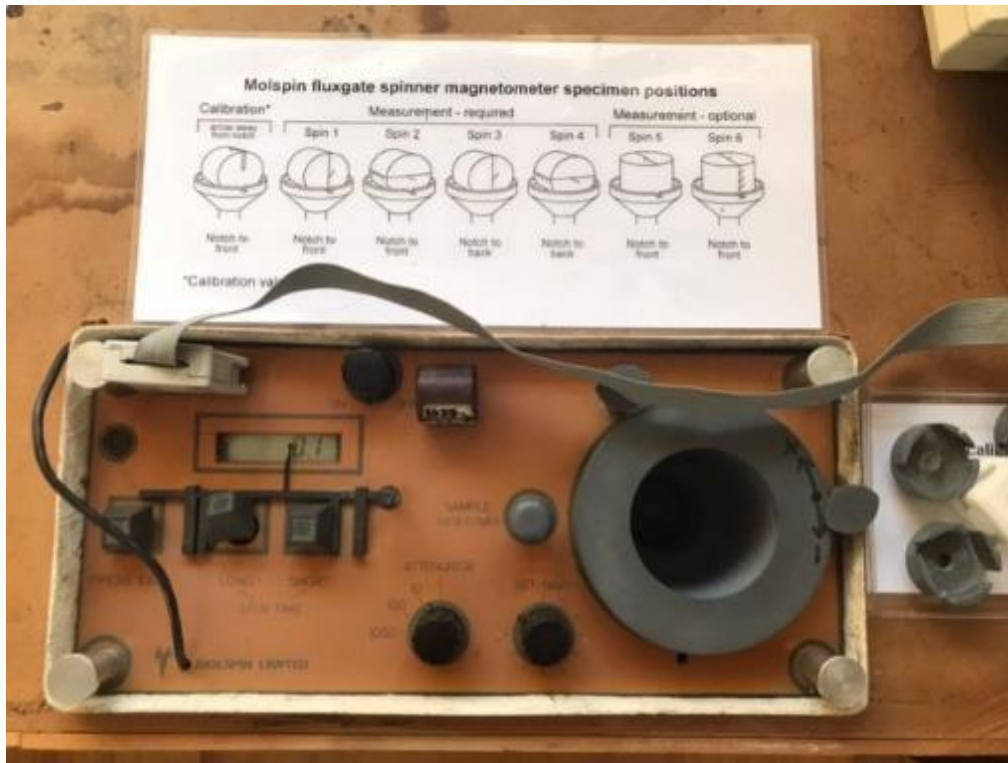
Figure 3.22. Molspin fluxgate spinner magnetometer. The positions for calibration and measurements can be seen on the picture. The calibration and the first four spin positions were used for this study. For each specimen, the intensity, declination, and inclination values were calculated by the program.
