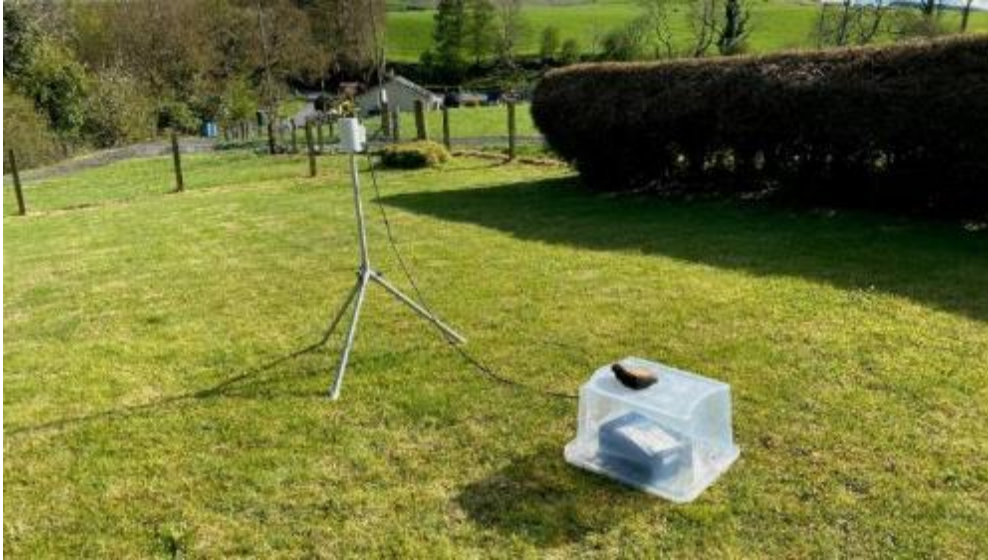
Figure 3.3. The base station was located away from human-made magnetic sources. The magnetometer of the base station was put into a plastic box to protect it from rain.
