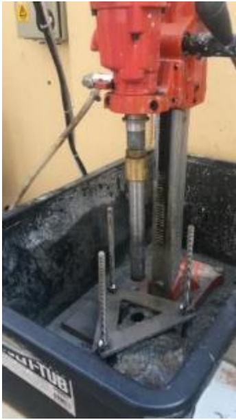
Figure 3.17. Left: Drilling machine used to obtain cores from hand samples. Right: Palaomagnetic saw for cutting cores to get the specimens. The distance between the blades was selected as 21 mm to obtain a suitable specimen for measurements. These specimens were used in the AGICO KLY-5 Kappabridge for anisotropy of magnetic susceptibility (AMS) measurements and the Molspin fluxgate spinner magnetometer for Natural remanent magnetization (NRM) measurement.
