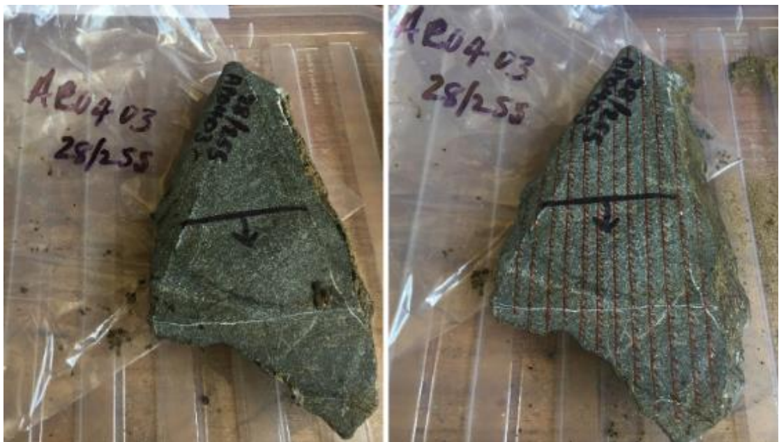
Figure 3.16. Left: An oriented hand sample, dolerite, was collected from site four. Dip and dip direction notes were written on the left corner. Right: The same sample after preparation for drilling. Red lines were plotted perpendicular to the strike and arrows showing the up-dip direction.
