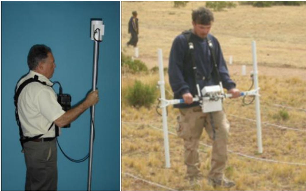
Figure 2.16. Left: A proton precession magnetometer (from GEOMETRICS, 2014). Right: A Fluxgate magnetometer (from Ernenwein and Hargrave, 2007).
