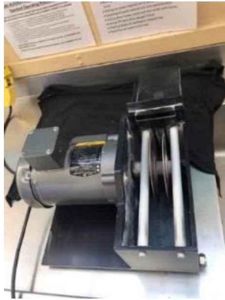
Figure 3.17. Left: Drilling machine used to obtain cores from hand samples. Right: Palaomagnetic saw for cutting cores to get the specimens. The distance between the blades was selected as 21 mm to obtain a suitable specimen for measurements. These specimens were used in the AGICO KLY-5 Kappabridge for anisotropy of magnetic susceptibility (AMS) measurements and the Molspin fluxgate spinner magnetometer for Natural remanent magnetization (NRM) measurement.
