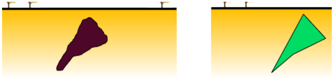
Figure 3.27. An irregular-shaped body in the subsurface is shown on the left side. The approach, using a multi-sided polygonal prism with straight sides, is shown on the right (from Morris, 2020).
