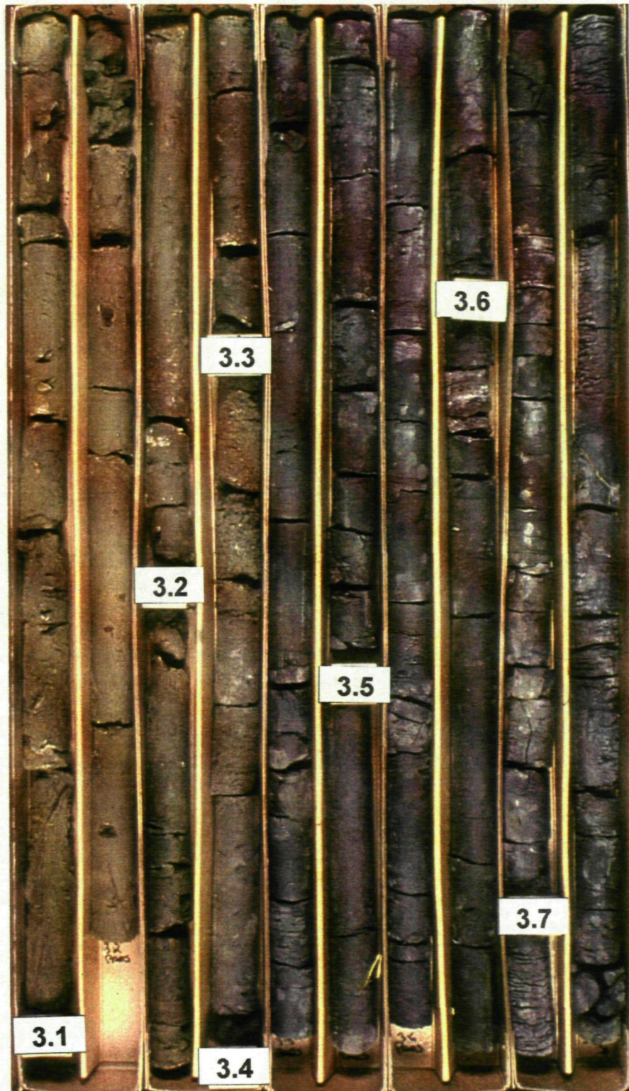
Figure 3.2. Hallett's Farm Borehole core photographs. Cores 3.1 to 3.8 ( pars ). The core numbers are situated at the base of each core and represent the following depths. Core 3.1 – 2.91m, 3.2 – 4.43m, 3.3 – 5.95m, 3.4 – 7.47m, 3.5 – 8.99m, 3.6 – 10.51m, 3.7 – 12.03m. (NB. In this Figure and all subsequent Figures depicting core photographs, the core box length = 1m).
