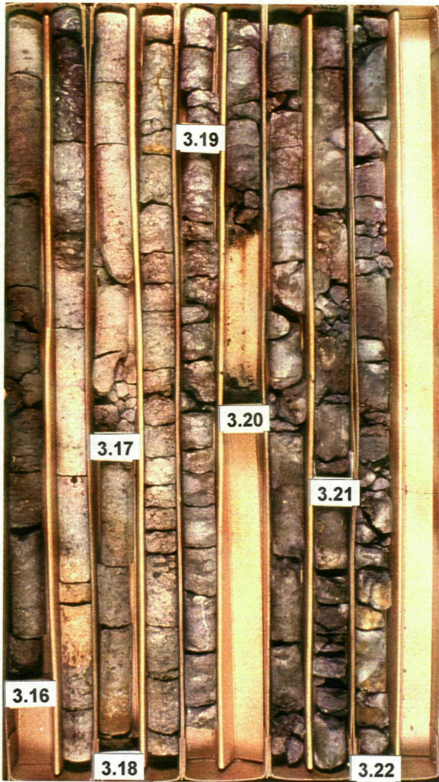
Figure 3.4. Hallett's Farm Borehole core photographs. Cores 3.16 ( pars ) to 3.22. The core numbers are situated at the base of each core and represent the following depths. Core 3.16 – 24.58m, 3.17 – 26.27m, 3.18 – 26.75m, 3.19 – 27.95m, 3.20 – 29.26m, 3.21 – 30.94m, 3.22 – 32.25m.
