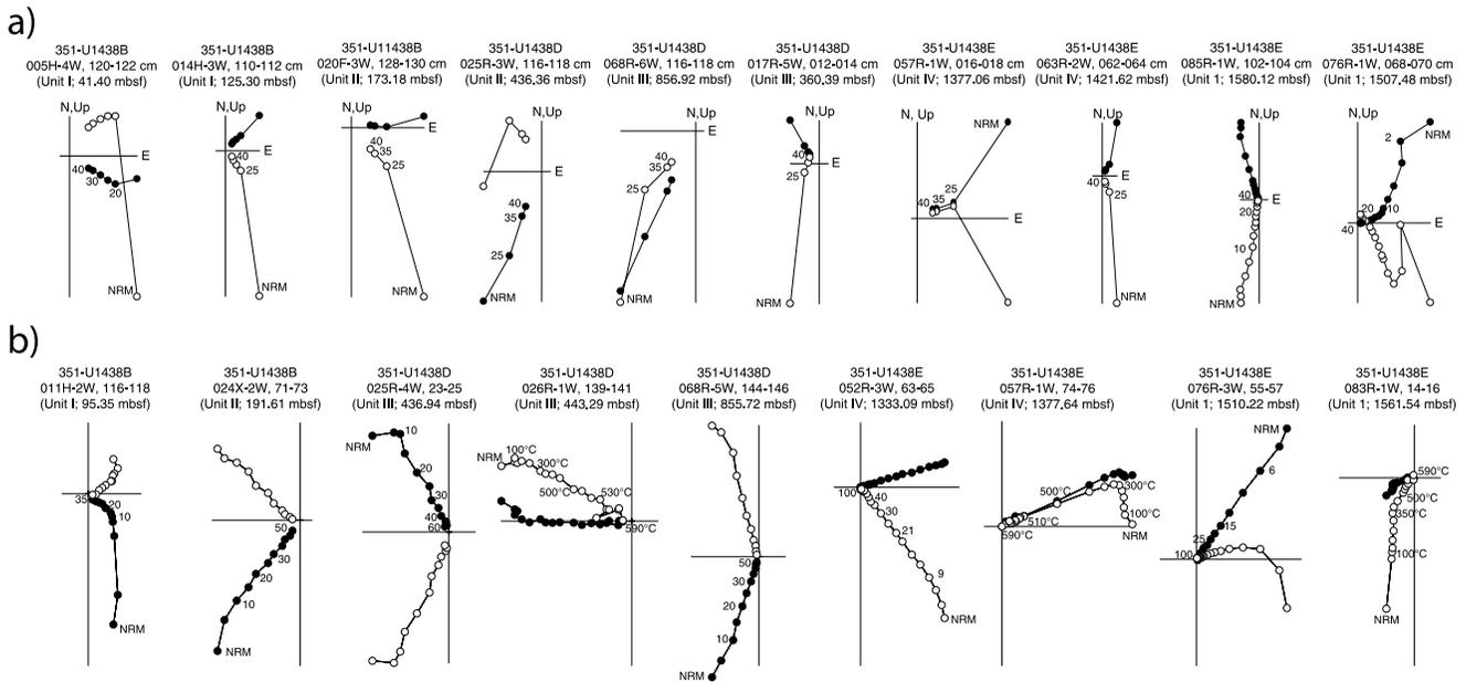
**Figure 2.** Representative demagnetization plots from (a) half core sections and (b) discrete specimens. Solid (open) dots are the projection on the horizontal (vertical) plane. Demagnetization steps in milliTesla (mT) or in °C are indicated in each plot.
