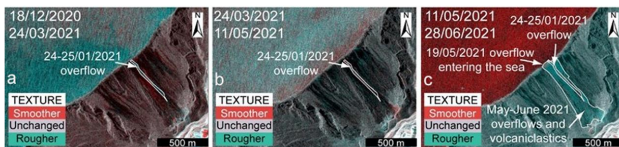
Figure 7. RGB colour composite of amplitude CSK images: (a) 24 March 2021–18 December 2020; (b) 25 May 2021–24 March 2021; (c) 28 June 2021–25 May 2021.
