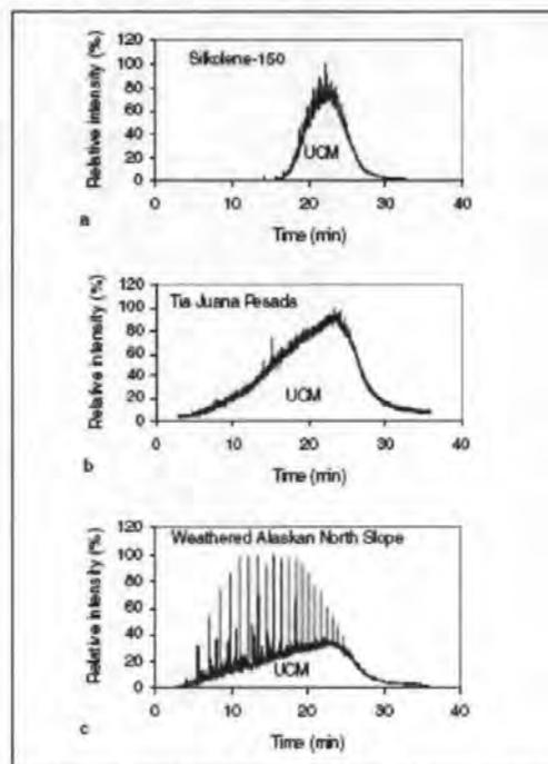
Fig. 1: Gas chromatograms of whole oils showing the unresolved complex mixture (UCM) of hydrocarbons
