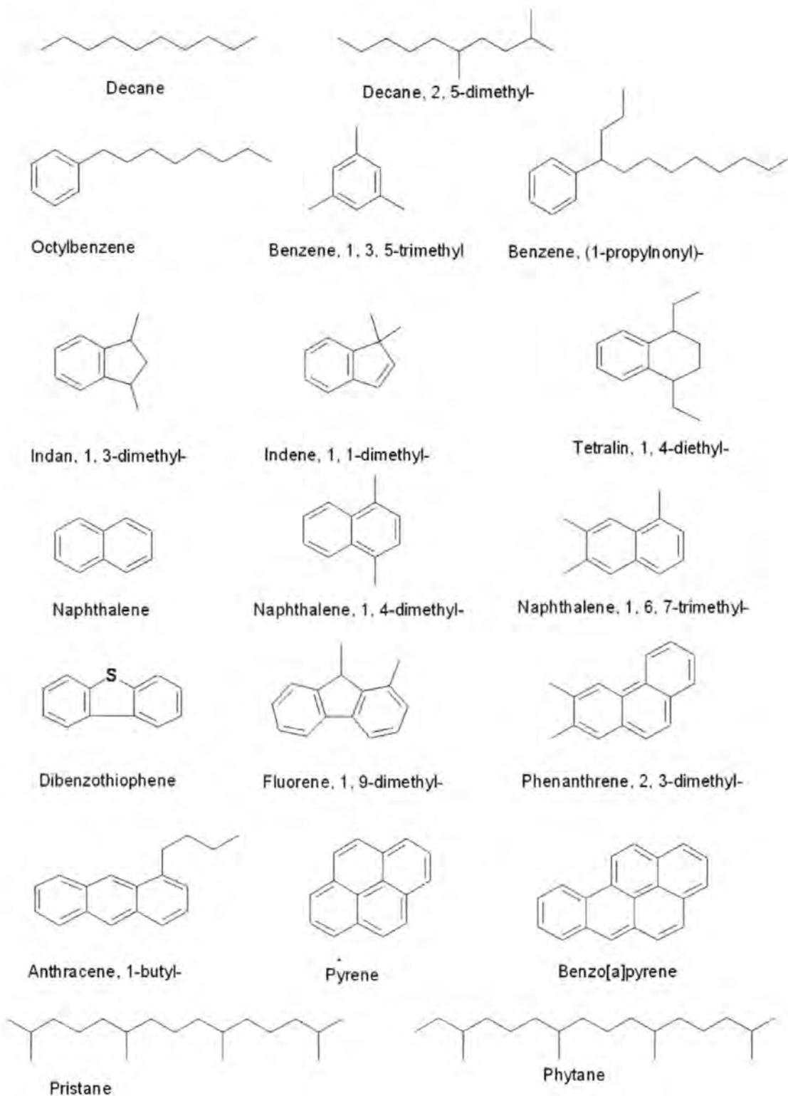
**Figure 1.1** Examples of aliphatic and aromatic hydrocarbons, including some alkylated compounds, commonly found in the environment that can normally be resolved by gas chromatography.
