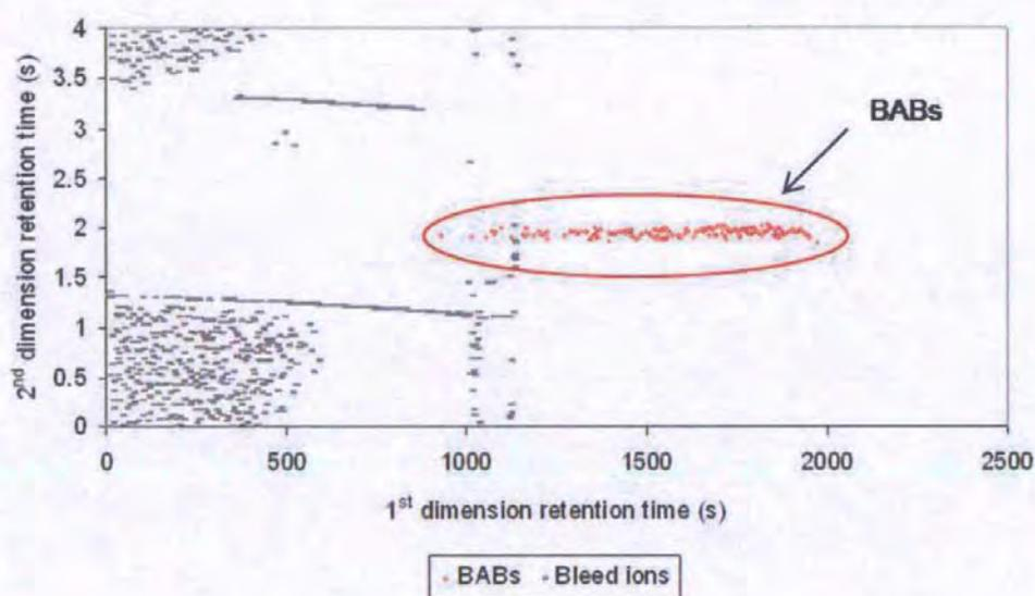
**Figure 5.6** Chromatographic peak marker plot derived by GC×GC-ToF-MS analysis of a complex mixture of C<sub>12-14</sub> branched alkylbenzenes (BABs, 0.1 mg mL<sup>-1</sup>) showing band of alkylbenzenes distinct from the column bleed compounds.
