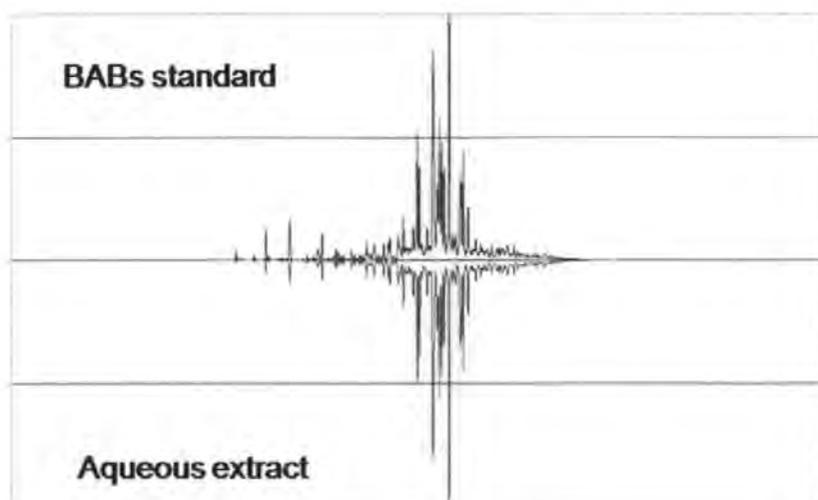
Figure 5.4 Comparison of a TIC of  $C_{12-14}$  BABs standard ( $1.0 \text{ mg mL}^{-1}$ , top) with TIC of aqueous extract at equivalent concentration (mirror image below).
