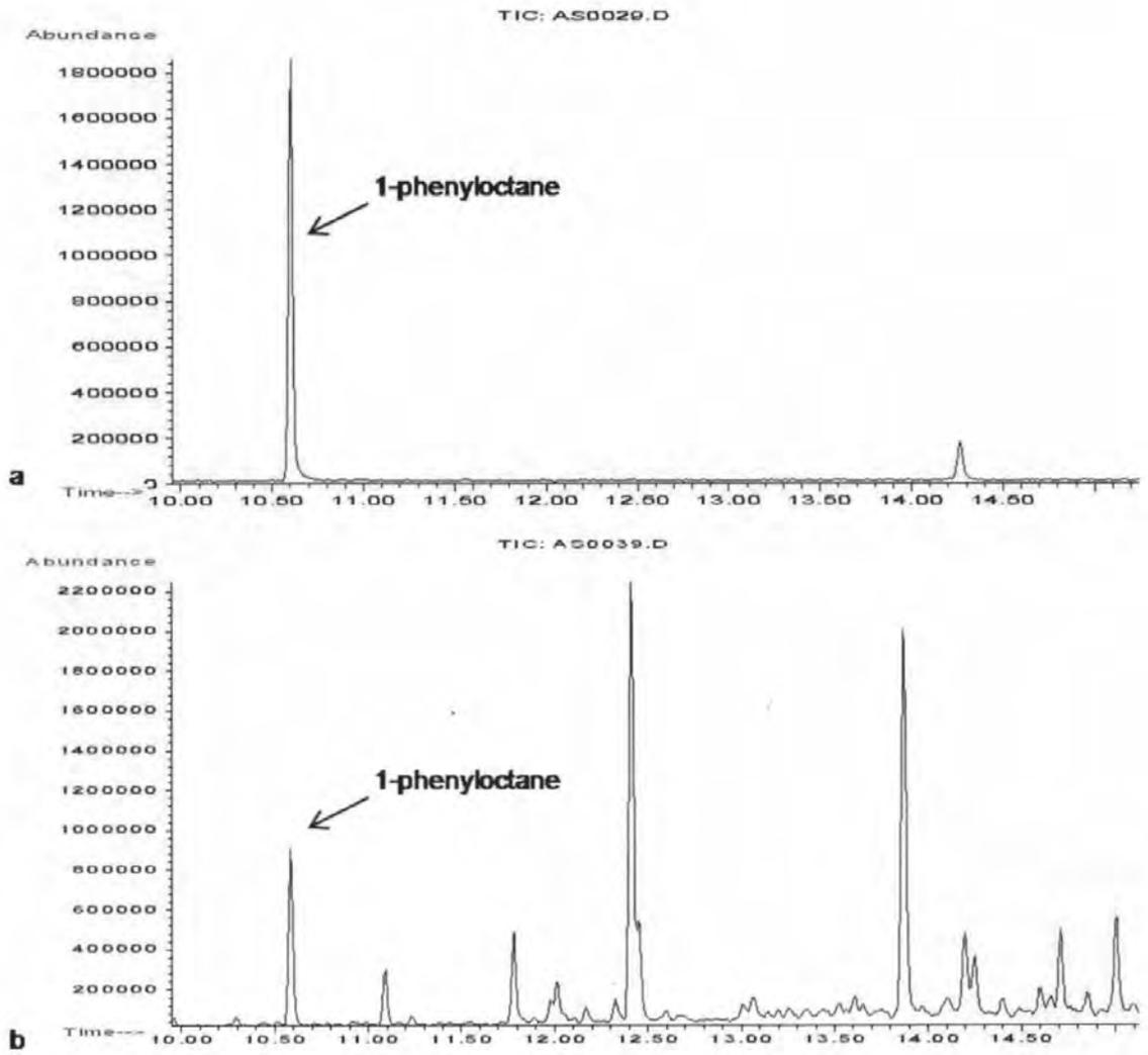
Figure 5.7 Total Ion Chromatograms of (a) 1-phenyloctane standard ( $0.005 \text{ mg L}^{-1}$ ) and (b) extract from mussels exposed to  $41 \text{ } \mu\text{g L}^{-1}$  1-phenyloctane.
