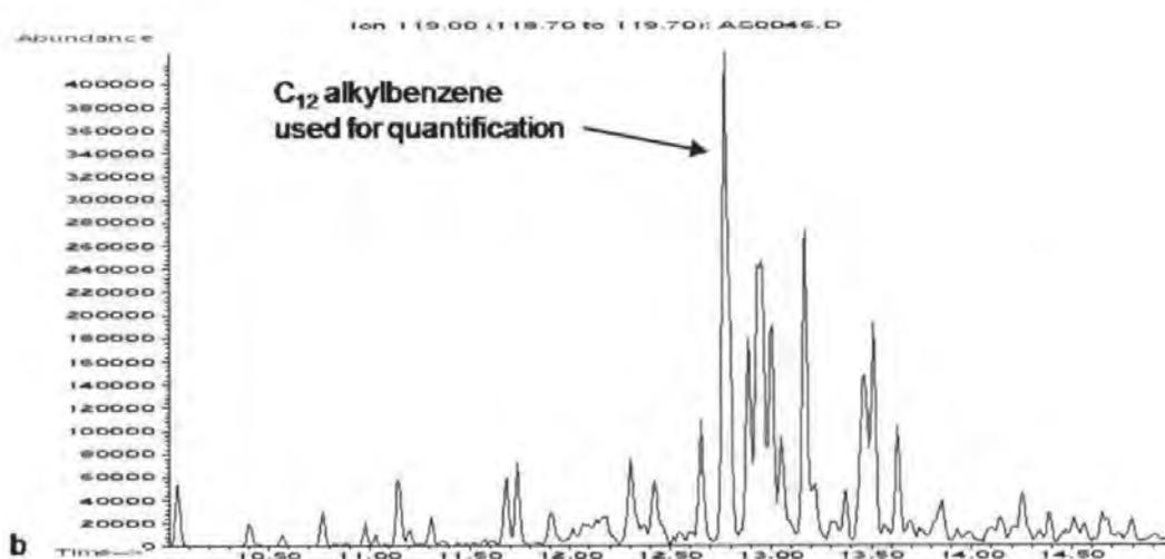
Figure 5.9 Chromatograms of common fragment ion  $m/z$  119 of (a) branched alkylbenzenes mixture of compounds standard ( $0.1 \text{ mg mL}^{-1}$ ) and (b) extract of tissues from mussels exposed to  $41 \text{ } \mu\text{g L}^{-1}$ .
