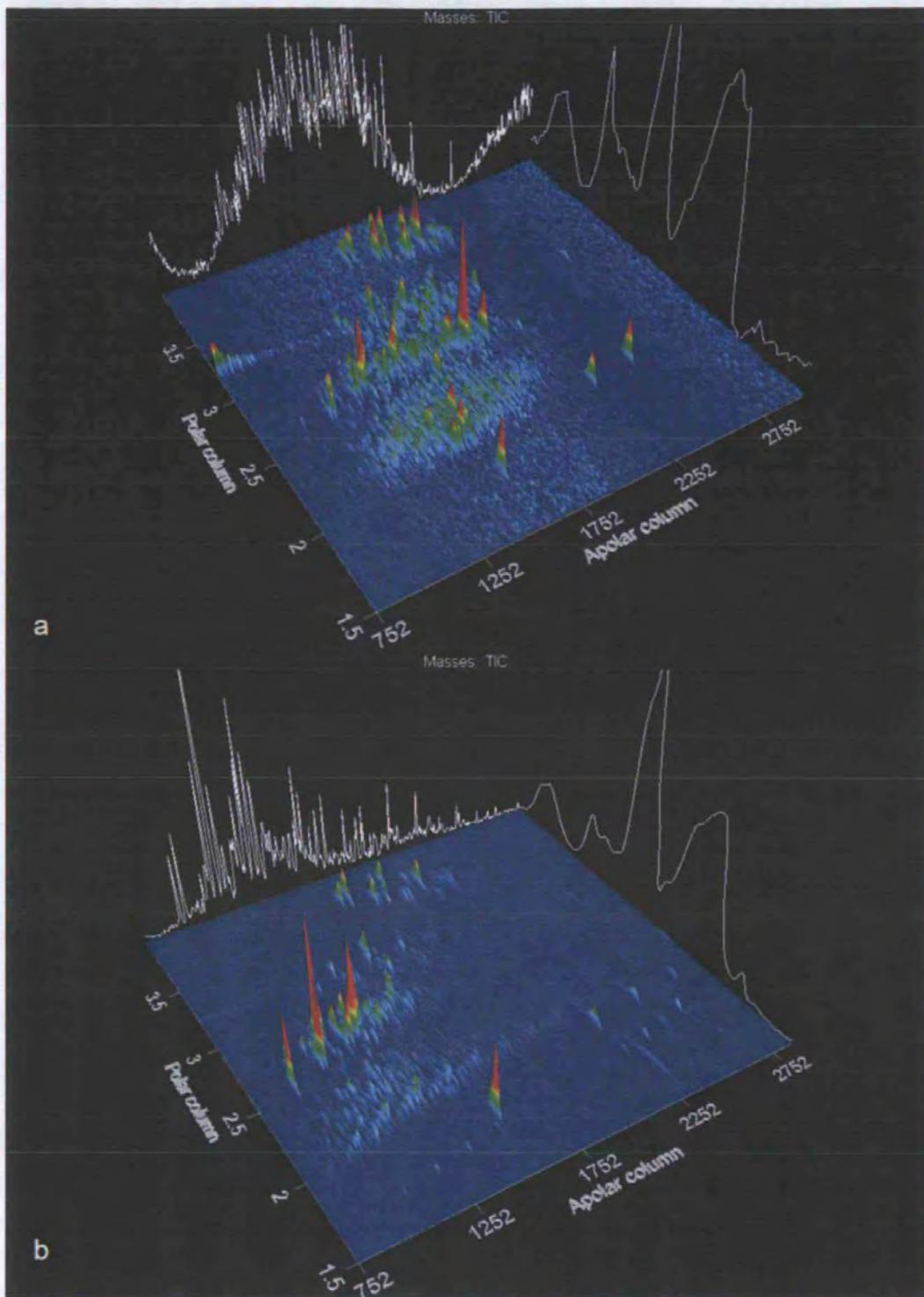
Figure 4.5 GCxGC-ToF-MS 3-D plots of F2 aromatic fractions of TJP (a) and ANS (b) oils. The chromatogram along the primary dimension axis (apolar) shows the typically UCM "hump" of conventional gas chromatograms.
