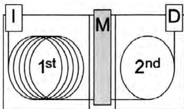
**Figure 1.3** Schematic of a GC×GC system. I, injector; M, modulator; D, detector; 1st, GC oven with first-dimension column; 2nd, separate, GC oven with second-dimension column. Reprinted from Dallüge *et al.* (2003).
