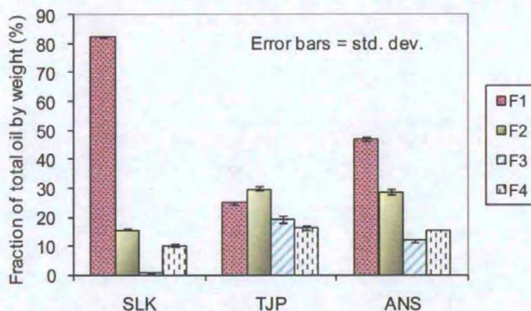
Figure 2.3 Gravimetric analysis of fractions of oils created by open column chromatography ( $n = 3$ ). F1 = aliphatic fraction eluted by 100 % hexane; F2 = aromatic 1 fraction eluted by 90:10 (v/v) hexane:DCM; F3 = aromatic 2 eluted by 100 % DCM; and, F4 = polar fraction eluted by 100 % methanol.
