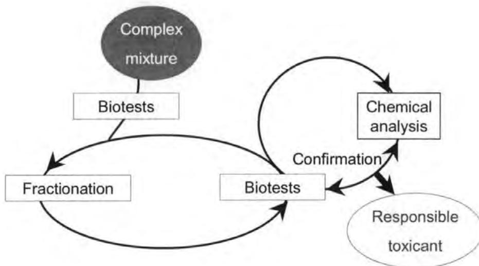
Figure 1.6 Scheme of effect-directed analysis of a complex mixture. Adapted from Brack (2003).
