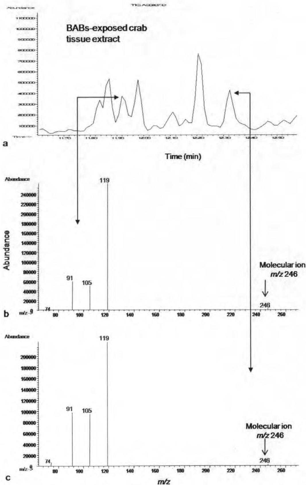
Figure 6.7 Gas chromatogram of extract from crab *C. maenas* midgut gland tissue (a), showing peaks used for identification and quantitation of BABs, with mass spectra of the compounds shown below (b and c).
