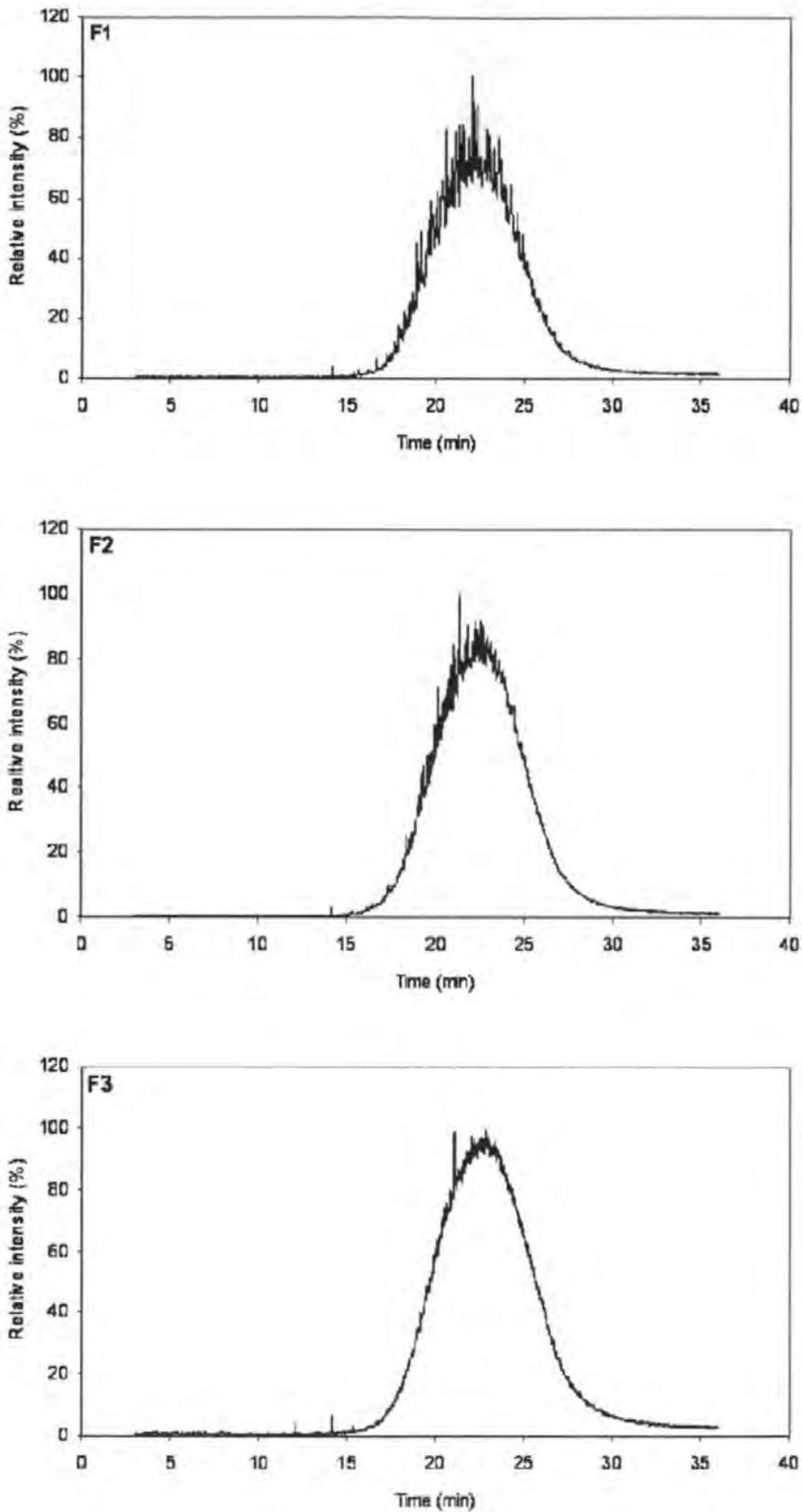
Figure 2.4 Gas chromatograms of fractions of Silkolene-150: aliphatic (top), aromatic 1 (middle) and polar aromatic 2 (bottom).
