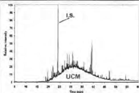
FIGURE 1. Total ion current gas chromatogram of the aromatic hydrocarbons extracted from mussels, *Mytilus edulis* sampled from Southend, U.K. I.S. = internal standard, 6,11-phenanthrene, 5  $\mu\text{g g}^{-1}$  dry mussel tissue<sup>-1</sup>; UCM = unresolved complex mixture; ca. 100  $\mu\text{g g}^{-1}$  dry mussel tissue<sup>-1</sup>.
