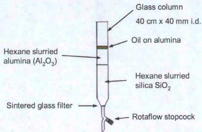
Figure 2.2 Apparatus used for large scale open column chromatography fractionation of oils.
