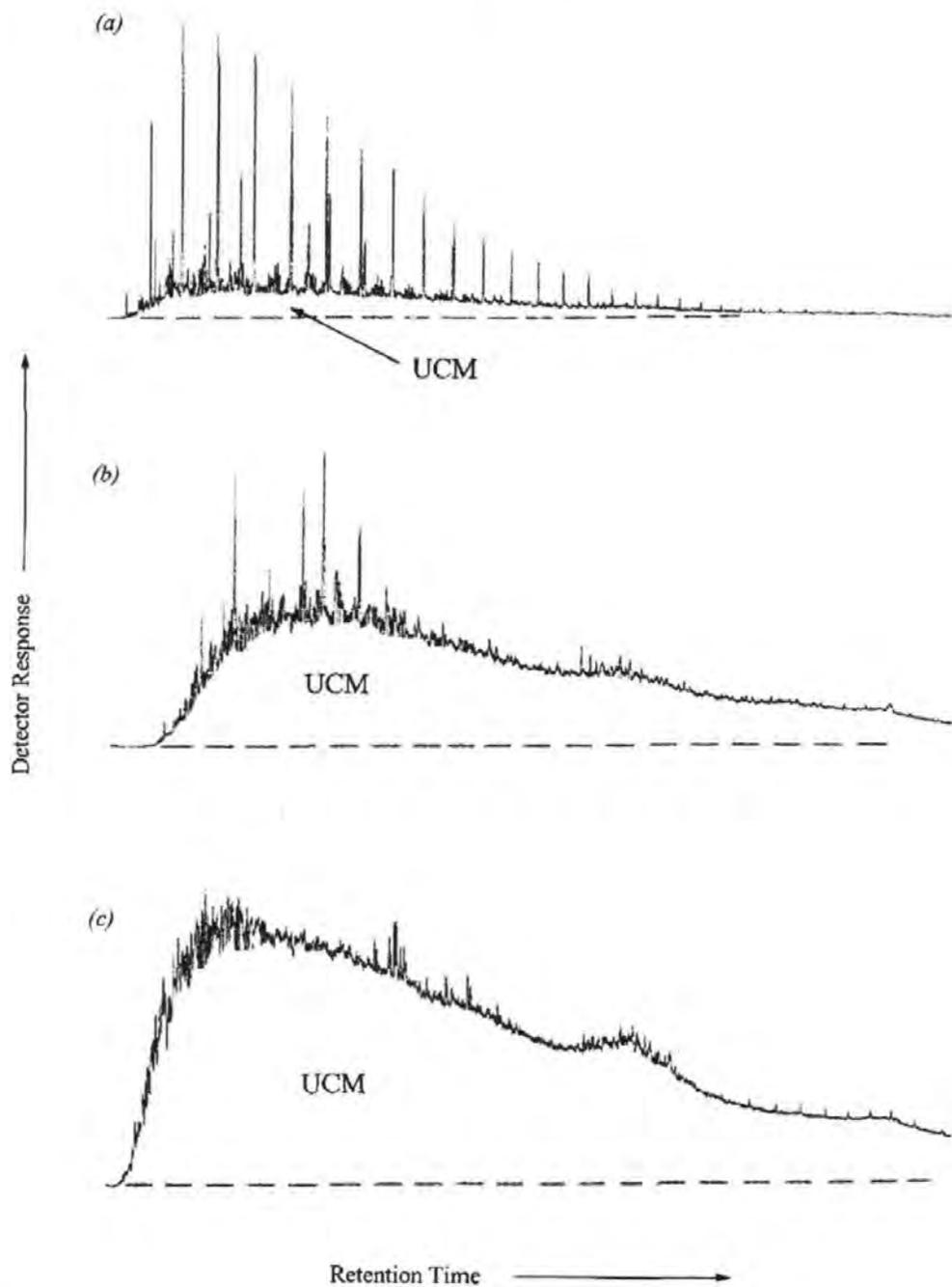
Figure 1.2 Gas chromatograms of three related Gulf Coast oils with differing levels of biodegradation: (a) nonbiodegraded; (b) moderately biodegraded; and, (c) very heavily degraded. Adapted from Peters & Moldowan (1993).
