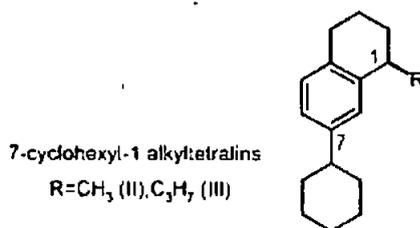
Figure 1.5 Example of disubstituted cyclic alkyltetralin. Reproduced from Smith *et al.* (2001).
