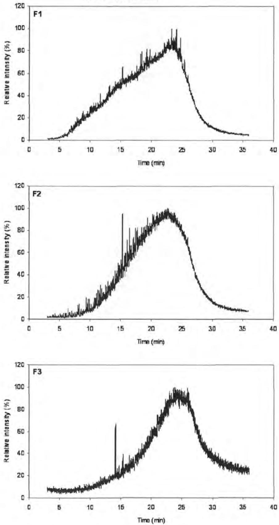
Figure 2.5 Gas chromatograms of fractions of Tia Juana Pesado: aliphatic (top), aromatic 1 (middle) and polar aromatic 2 (bottom).
