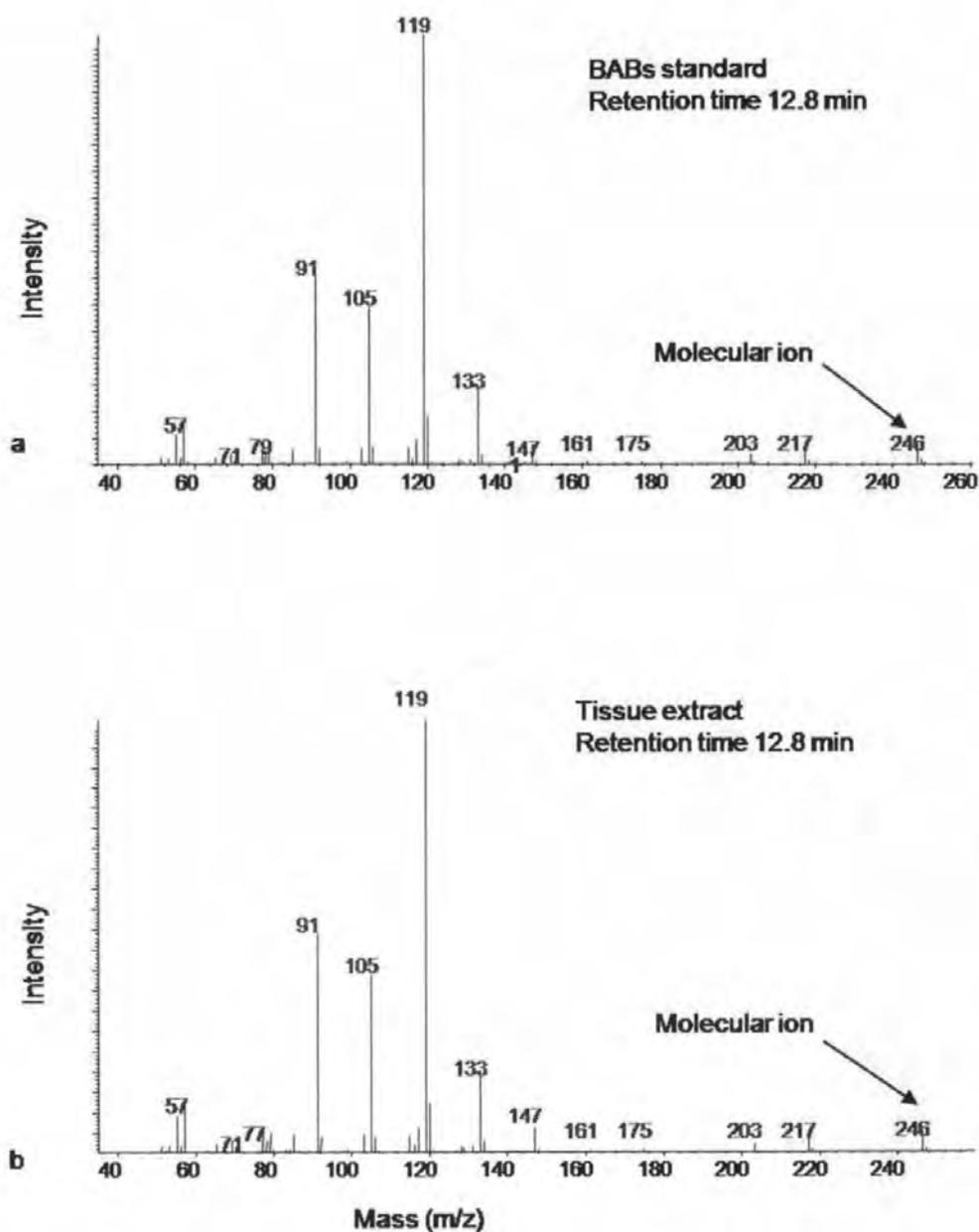
Figure 5.10 Mass spectra of peak at 12.8 min used for quantification of concentrations in mussel tissue extracts: (a) branched alkylbenzenes mixture of compounds standard ( $0.1 \text{ mg mL}^{-1}$ ) and, (b) extract of tissues from mussels exposed to  $41 \text{ } \mu\text{g L}^{-1}$ .
