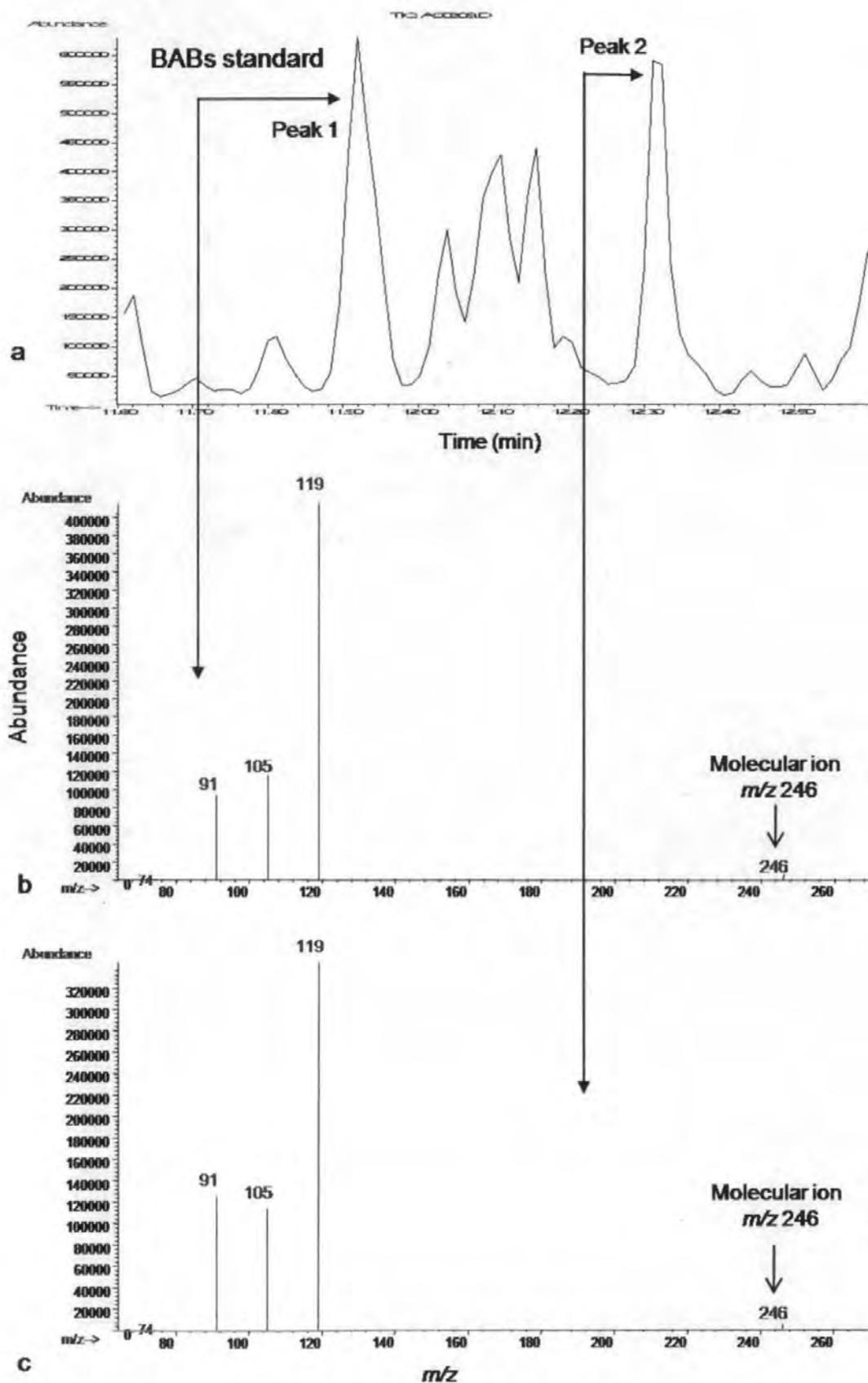
Figure 6.6 Gas chromatogram of C<sub>12-14</sub> BABs mixture standard (a), showing peaks used for identification and quantitation of BABs in crab tissue, with mass spectra of the compounds shown below (b and c).
