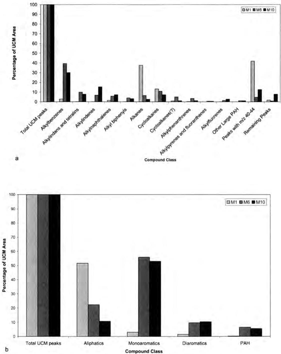
**Figure 1.4** Structural classes of hydrocarbons (a) and more general classes (b) of compounds derived by tandem gas chromatography analysis of three UCMs that elicit high (M1), medium (M6) and low (M10) Scope for Growth (a measure of the capacity for growth and reproduction) in *Mytilus edulis*. Graphs and data republished from Booth *et al.* (2006).
