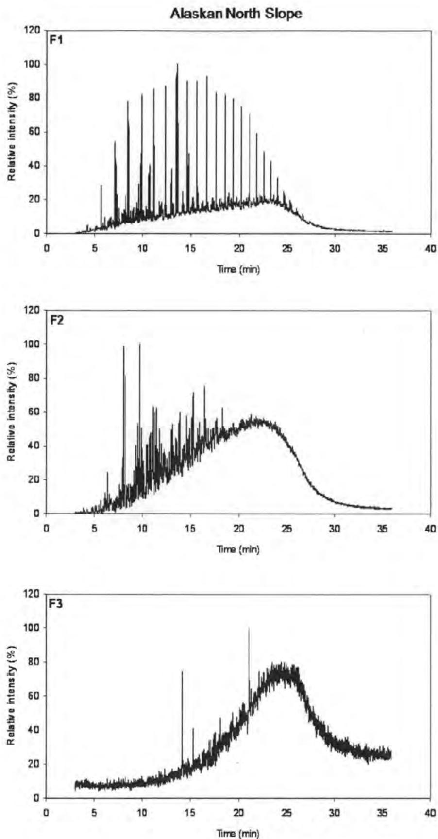
Figure 2.6 Gas chromatograms of fractions of weathered Alaskan North Slope: aliphatic (top), aromatic 1 (middle) and polar aromatic 2 (bottom).
