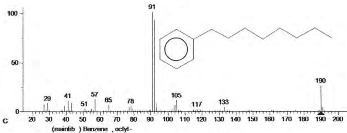
Figure 5.8 Mass spectra of peak at 10.6 min (a) 1-phenyloctane standard ( $0.005 \text{ mg mL}^{-1}$ ), (b) extract from mussels exposed to  $41 \mu\text{g L}^{-1}$  1-phenyloctane and (c) NIST library 1-phenyloctane.
