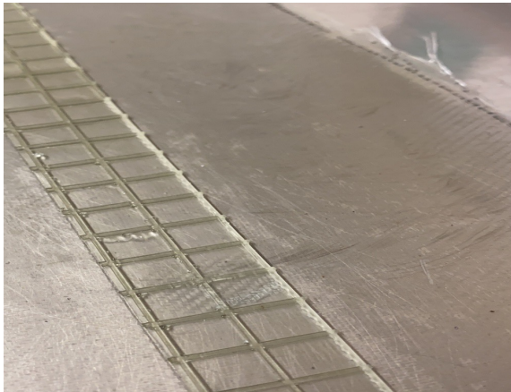
Fig. 5: REFLOW reusable flow aid illustrates resin moulded witness 1mm section used for intricate zones
