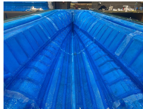
Fig. 4: MicroMorph lines provide reusable flow fields eliminating flow mesh
