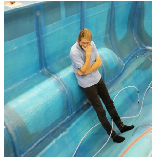
Fig. 3: Large reusable membrane with reusable resin feed channels
