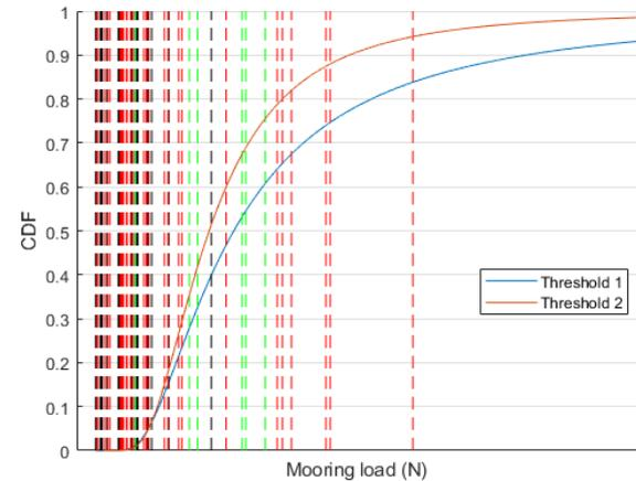
Fig. 9. CRRW, CNW, EVD comparison. CNW responses are given by red dashed vertical lines, CRRWs black and the 6 empirical 1 in 3hr extremes from the long irregular waves are green. The EVD CDF for threshold 1 is given in blue, threshold 2 is given by the solid red curve. Threshold 2 uses a larger threshold. Force magnitudes have been obscured by removing the x axis values.
