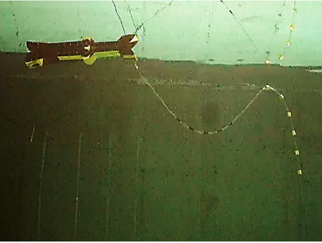
Fig. 1. Subsurface view of model WEC and Lazy S mooring line - experimental setup
