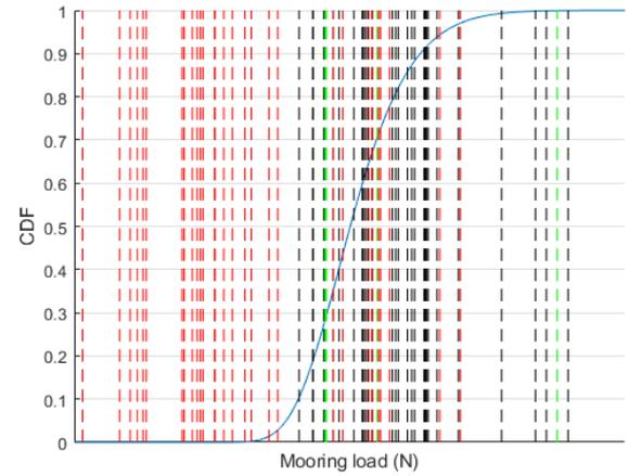
Fig. 11. CRRW CNW EVD comparison. CRRWs are black, CNWs red and the 4 empirical 1 in 3hr extremes from the long irregular waves are green. The EVD CDF is calculated based on the full scale equivalent of 12 hours of irregular waves. The x axis is obscured.
