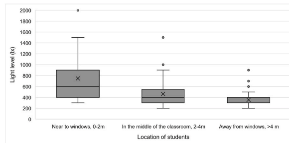
Fig. 15. Distribution of measured light level on students' desks in relation to the distance to windows.
