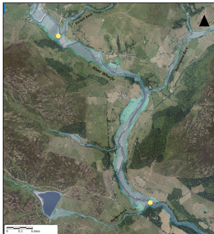
Figure 5-8 1 in 100 year (purple) and 1 in 1000 year (blue) flood map as shown for the study site on the River Wharfe
