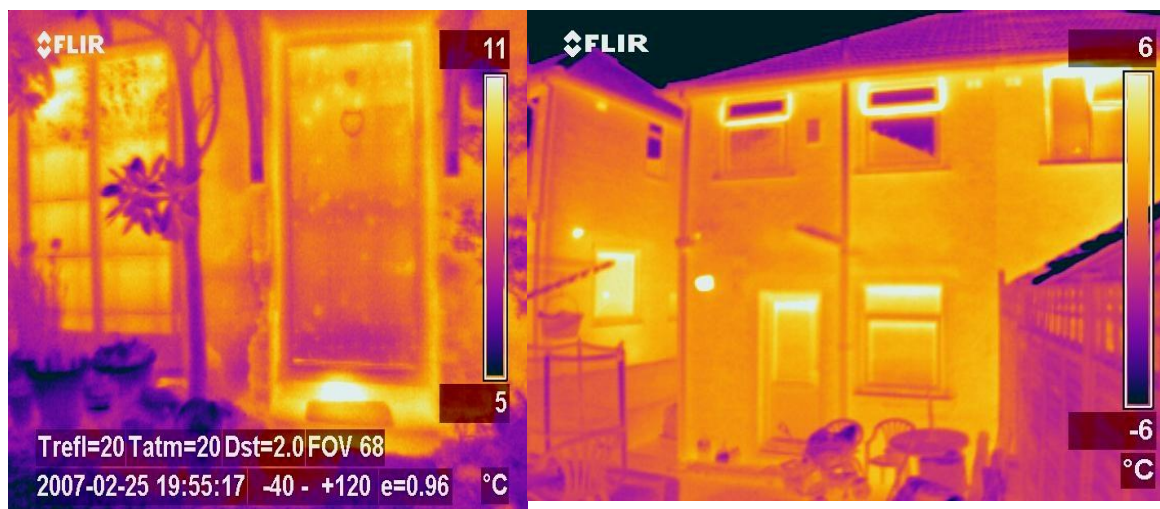
Figure 4.2: Thermal image example of two visible actions (draught proofing and closing windows when the heating is on).
