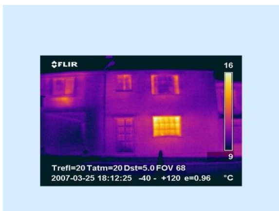
Figure 7.3: Thermal image showing a single glazed window.
