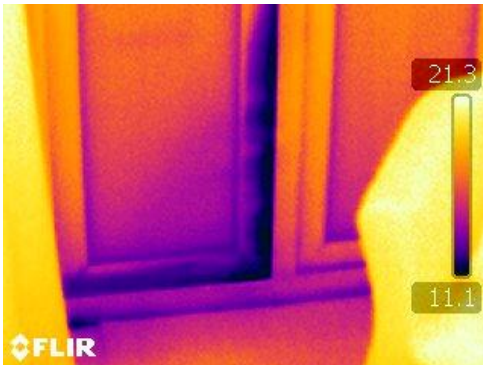
Figure 6.3: Example thermal image showing dark (cold) areas where there is cold air ingress around the surround of the doorway.
