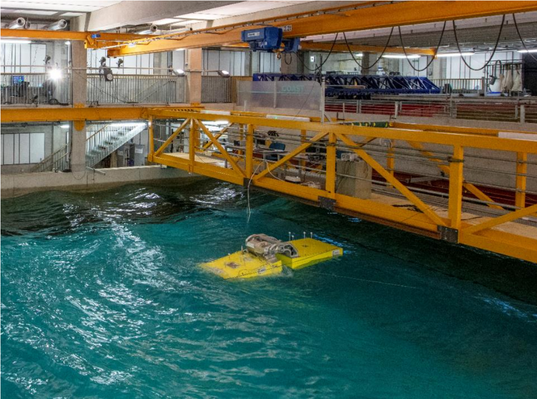
Figure 5.18: 1:25 hinged-raft model testing process in the wave basin.
