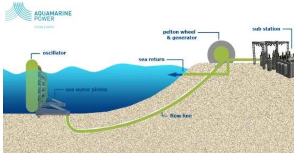
Figure 2.7: The general arrangement of the Oyster WEC system [23].
